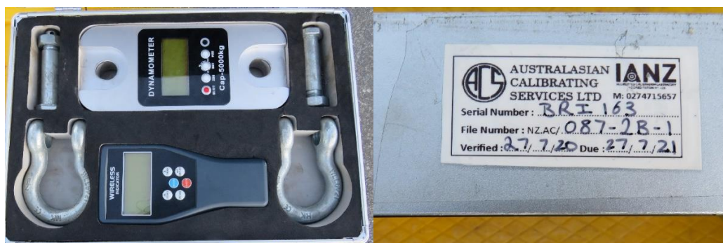
Figure 2: Load cell used for testing
