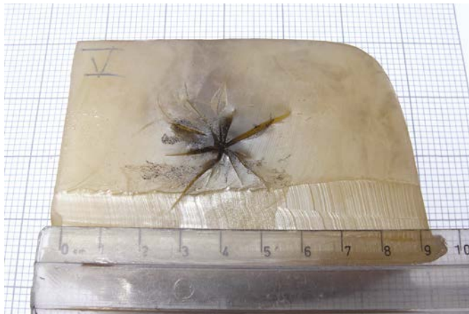
Figure 4.12: Axial view. Corbin's gel. 18 kV. (19,8 kA). Temporary cavity formation demonstrated in the harder gelatine media. Large fissure fracture noted similar to that seen in projectile testing experiments. The current strength measured 19,80 kA.
