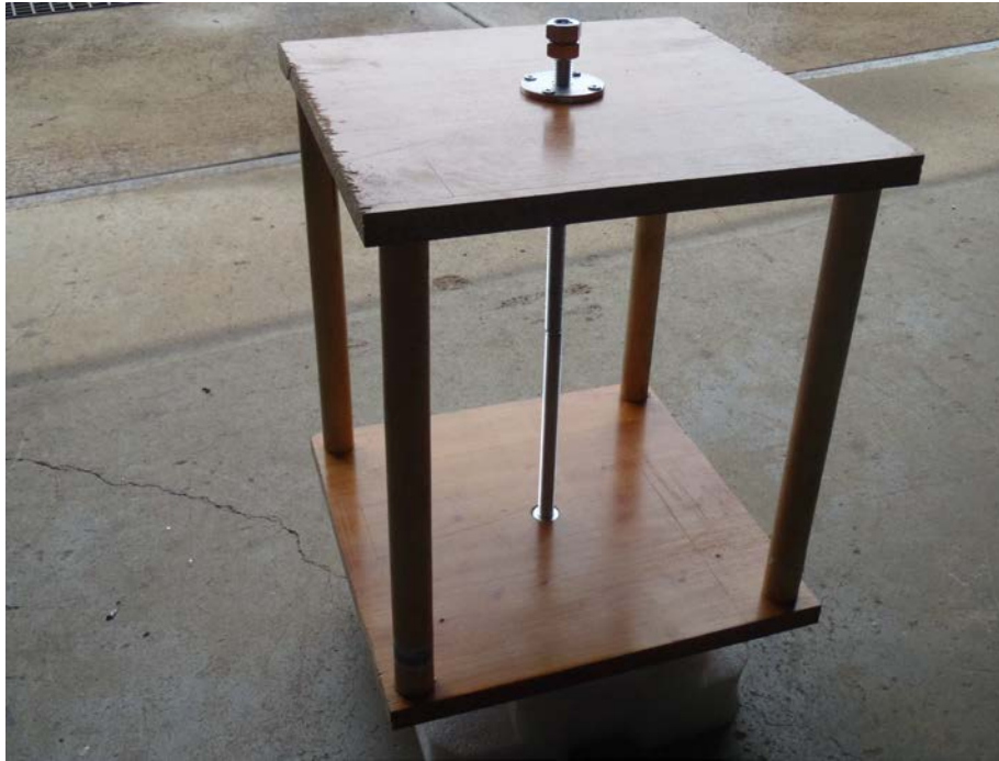
Figure 4.15: The test box, specifically constructed to create a spark gap of 5mm.
