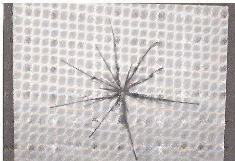
Figure 4.3: Axial view in the direction of the gunshot. Gelatine block with a gunshot (Sellier & Kneubuehl, 1994).
