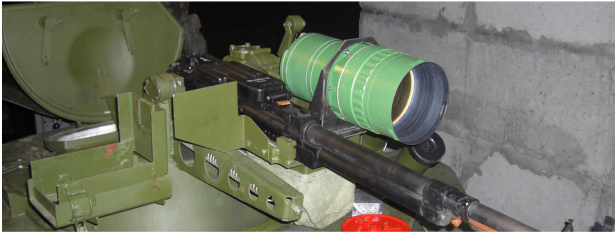
FIGURE 1: CYCLONE THERMAL IMAGING SYSTEM ON ARMORED VEHICLE TURRET
