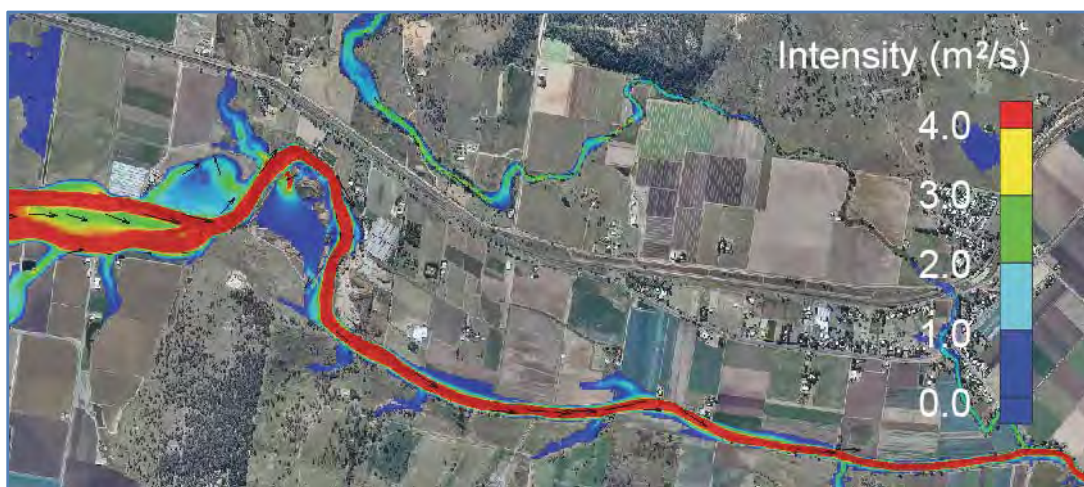
Figure 5.13: Image of modelled water levels at 3:25 pm on 10 January 2011 Source: Exhibit 144, John Macintosh, Most likely scenario animation
