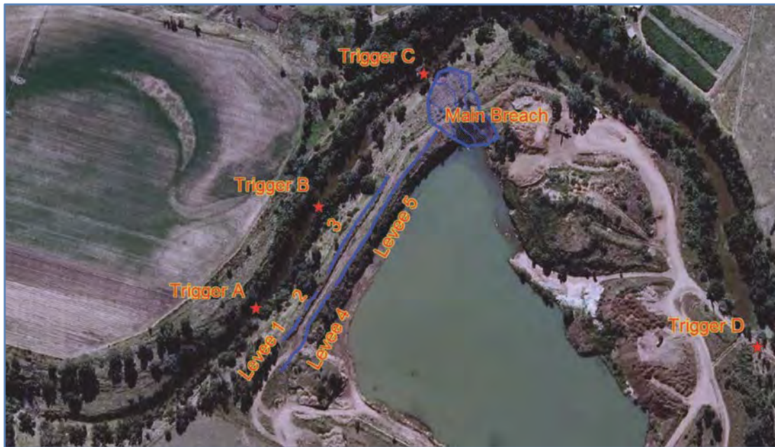
Figure C10 – Quarry failure trigger level locations
