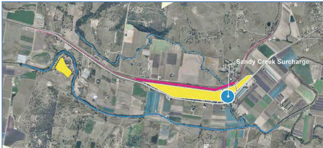
Figure 5.5: Diagram of first stage of flooding Grantham Source: Exhibit 144, Dr John Macintosh, Expert Hydrology Report – 10 January 2011 Flood – Circumstances and Contributing Factors , 11 August 2015 [p21: Figure 1.3(a)].
