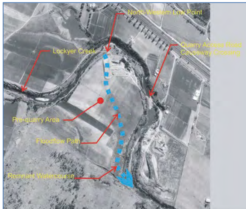
Figure C23: Quarry area in 1982 overlaid with flood path
