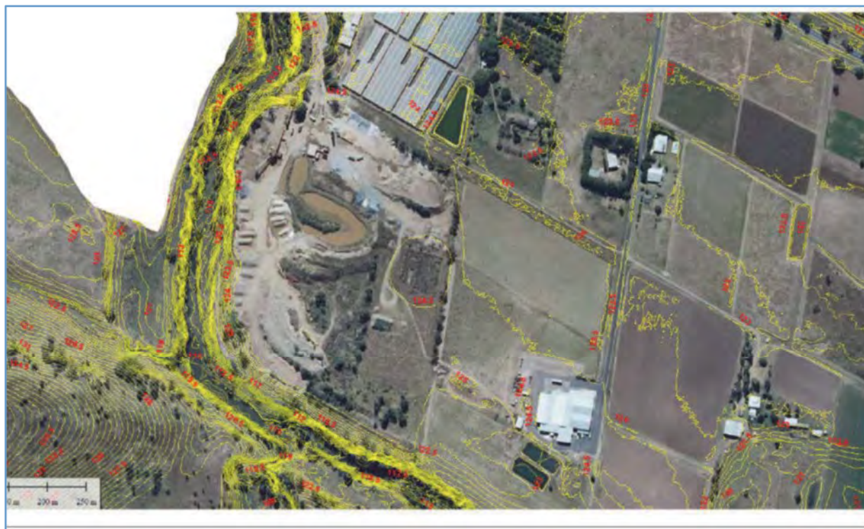
Figure A17: Reconstructed topographic plan of Batching Plant Site prior to development.
