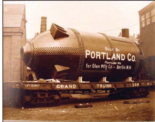
View of a Portland Company digester sitting between the Blacksmith & Tank shop and Boiler Shop. Courtesy of the Maine Historical Society.
