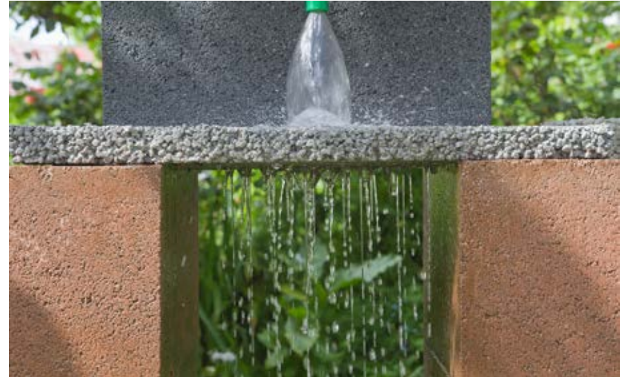
ABOVE: Permeable pavement has a lower amount of sand compared to conventional pavement, which allows water to quickly seep through to infiltrate into the ground below.
