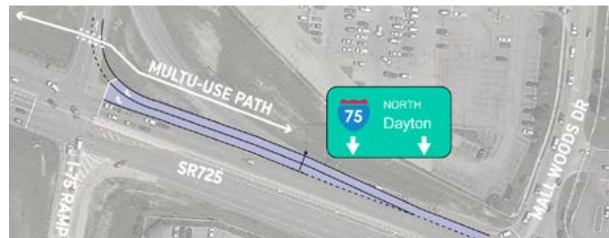
ABOVE: Installing dual right turn lanes on SR725 into the northbound I-75 ramp will improve lane utilization and improve pedestrian and bike safety if a multi-use path is placed on the north side of SR725
