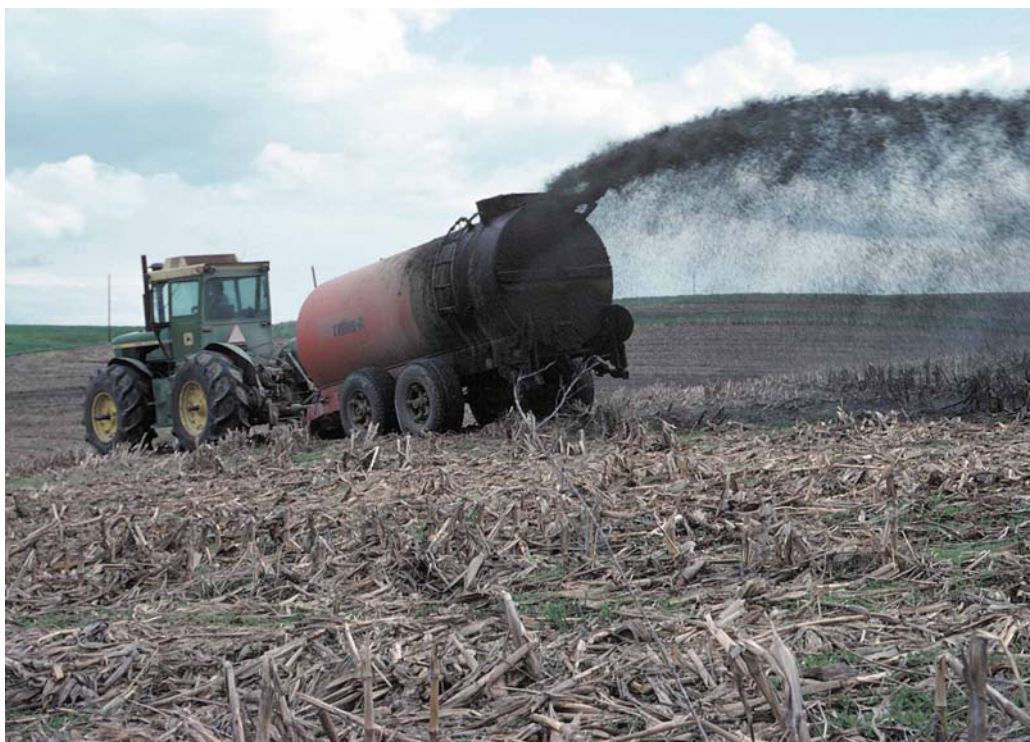
Figure 7.1. Tractor drawn liquid manure application after corn harvest.
