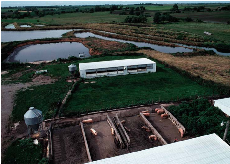
Figure 7.9. View of a hog operation with a lagoon flowing into constructed wetlands for treatment of wastewater.
