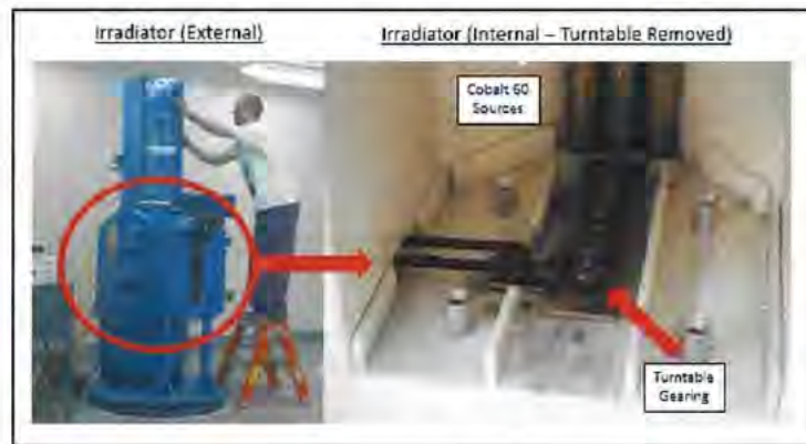
Figure 18: J&L Shepherd 484-R2 Gamma Irradiator at DPG-LSD
