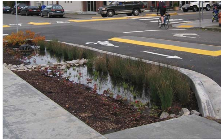
Bioswales within curb extensions create sustainable streets
