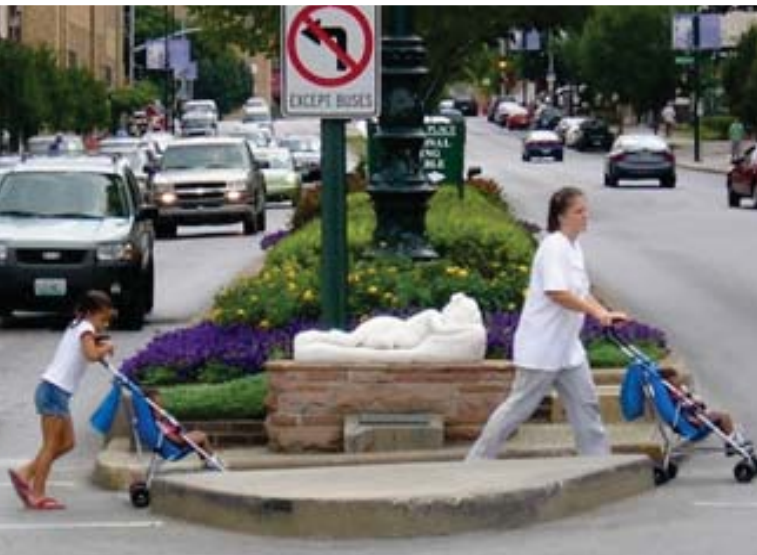
Medians provide pedestrian refuge mid-crossing
