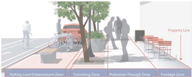
Elements of a Sidewalk Corridor Cleveland Complete and Green Streets Typologies Plan, 2013
