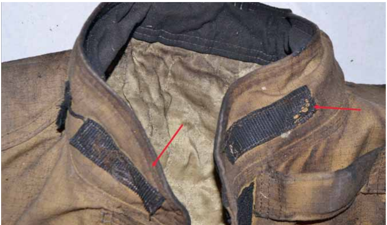
Figure 12: Neck area of coat showing cut/missing throat tab and thermal damage to Velcro loops on left side
