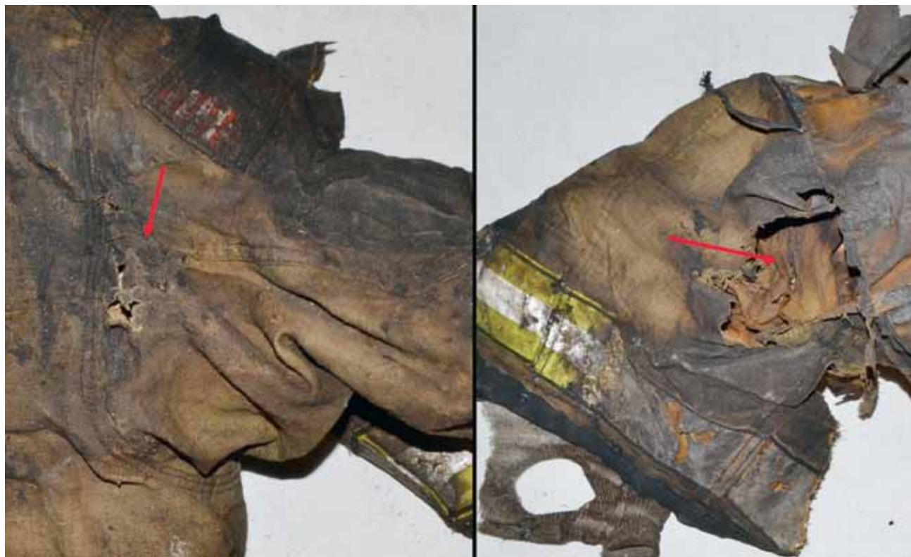
Figure 15: Thermal break open on both arms of coat
