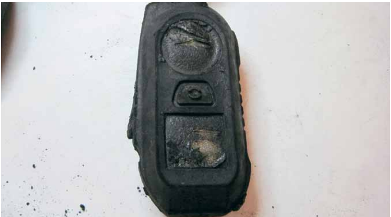
Figure 16: Significant heat damage to PASS console.
