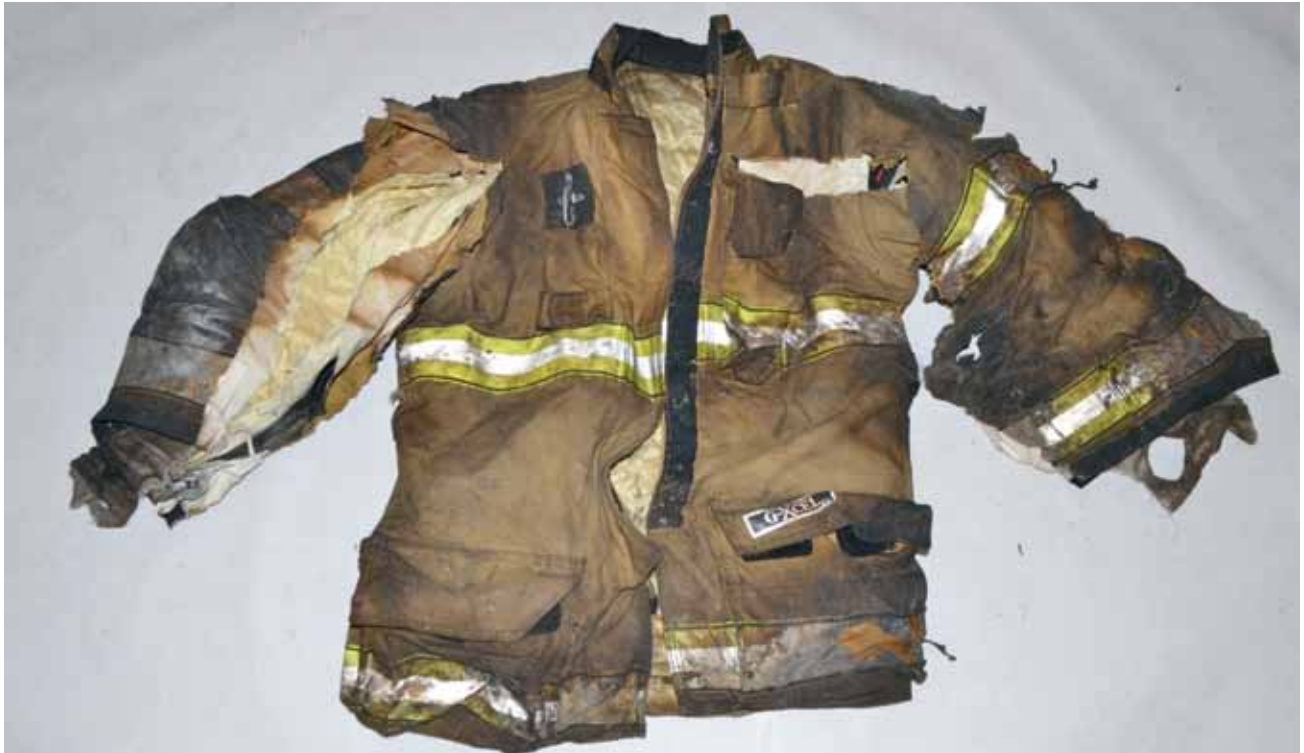
Figure 11: Front of coat showing cut areas and overall thermal damage to coat and reflective trim
