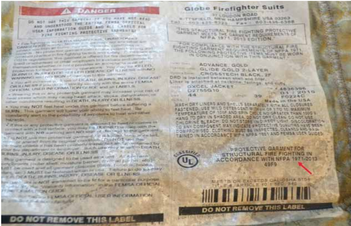
Figure 17: Label of coat showing NFPA certification and other garment information
