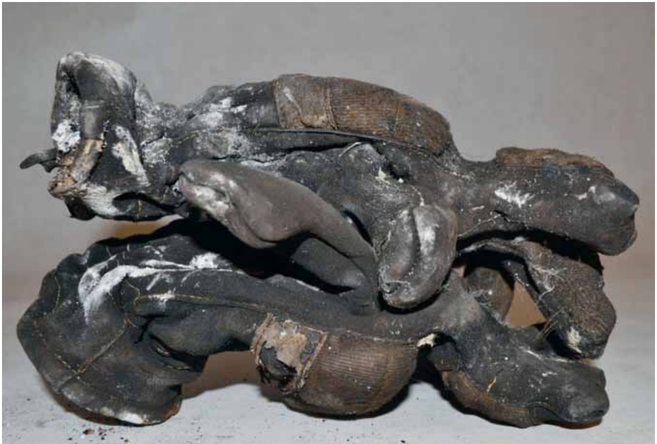
Figure 4: Alignment of the glove indentations suggest that the gloves were in a stowed position at time of incident
