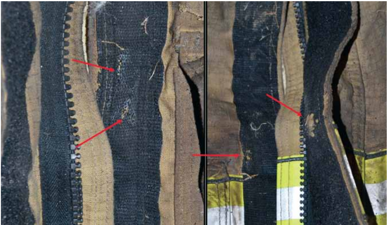
Figure 13: Melted areas on Velcro loops on inside of coat along the front zipper
