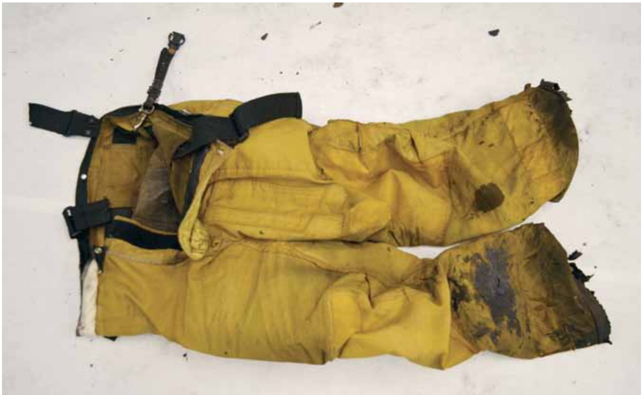
Figure 32: Outershell of pants turned inside-out showing thermal damage to lower leg and cuffs
