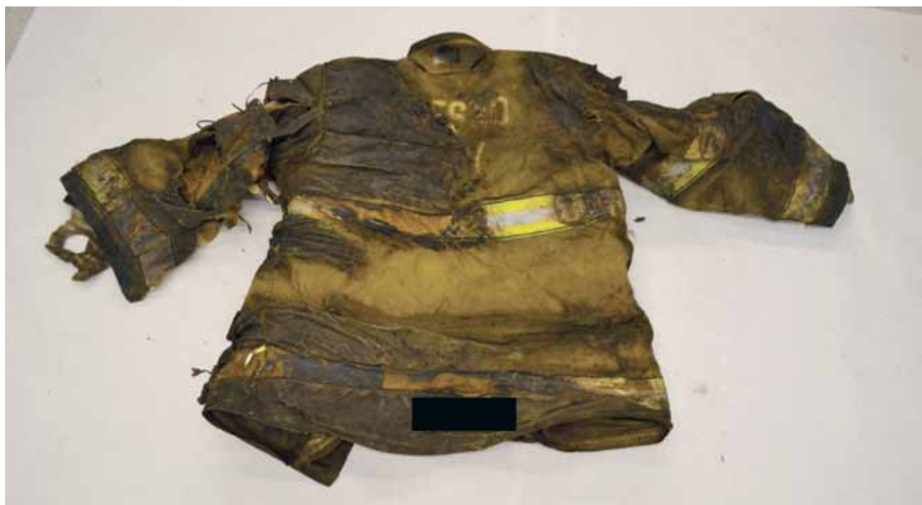
Figure 16: Substantial thermal damage on back left side of coat and reflective trim with clean area where the SCBA was positioned
