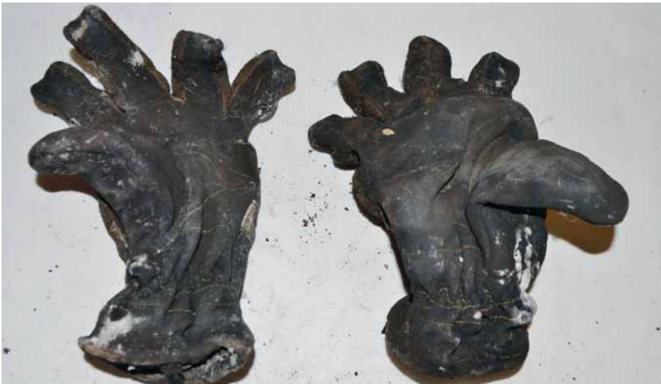
Figure 2: Palm side view of gloves with substantial thermal damage visible to outershell
