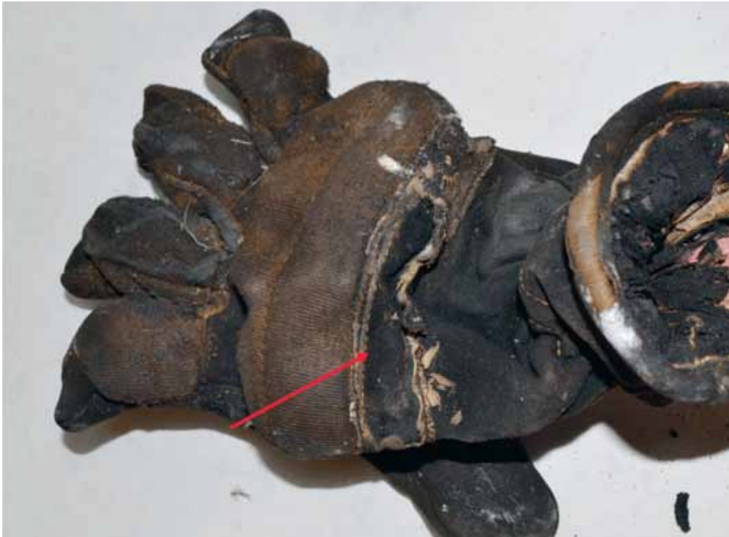
Figure 9. Thermal protective strip on back of right glove completely destroyed
