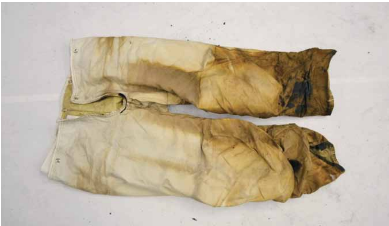
Figure 34: Moisture barrier side of pants liner showing thermal damage to cuffs
