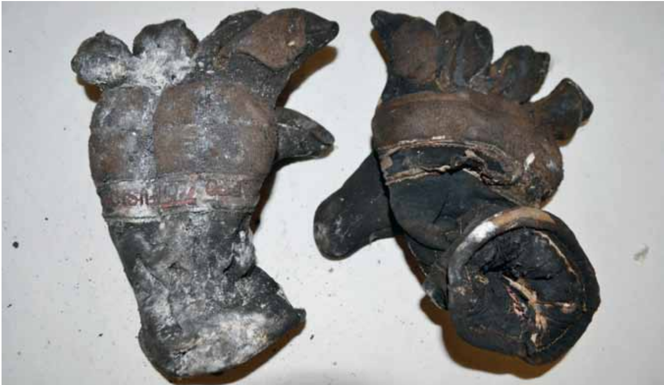
Figure 1: Top view of gloves with substantial thermal damage visible on outershell
