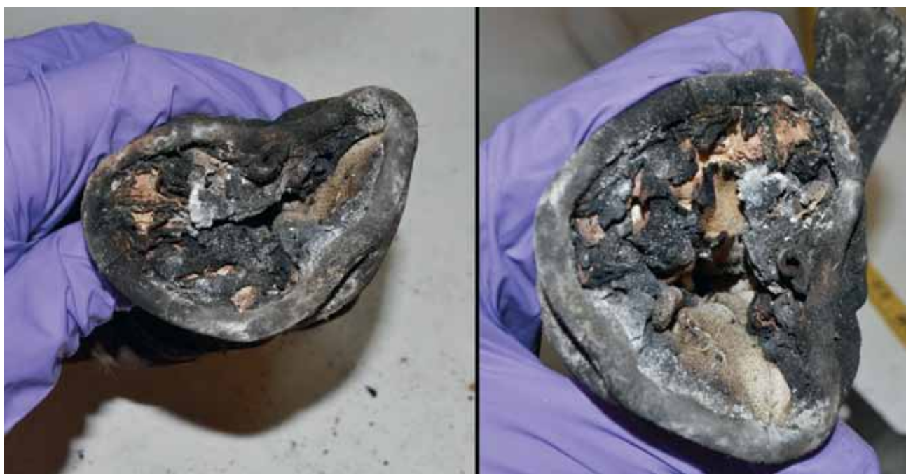
Figure 8: Break open on left glove at interface between liner and outershell
