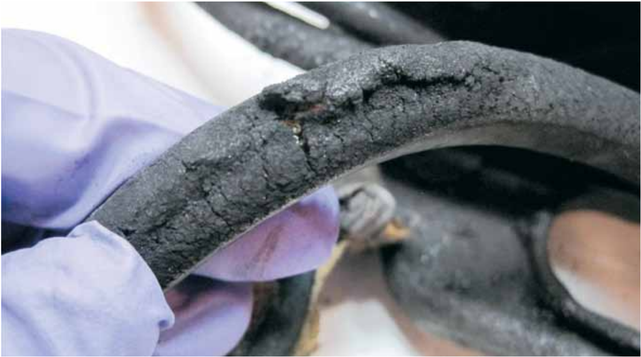
Figure 9: Low pressure hose possibly compromised.
