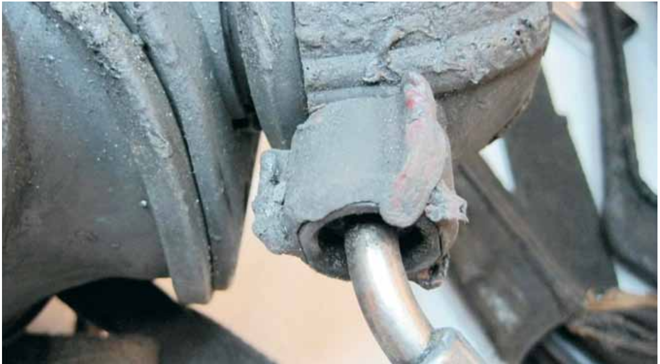
Figure 7: Melted bypass knob.
