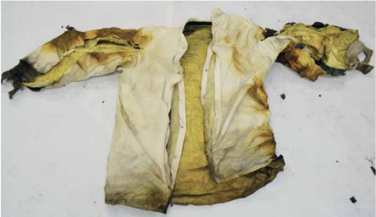
Figure 21: Substantial thermal damage to moisture barrier side of coat liner and visible cuts to both arms
