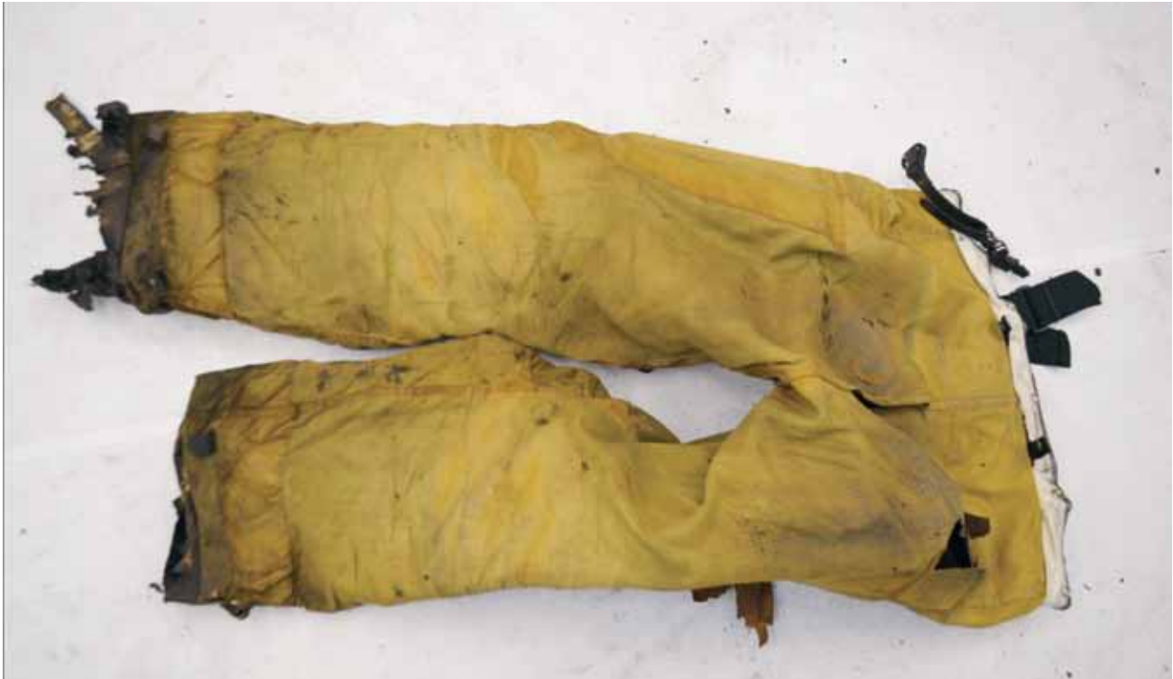
Figure 33: Outershell turned inside-out showing thermal damage to seat and cuff areas
