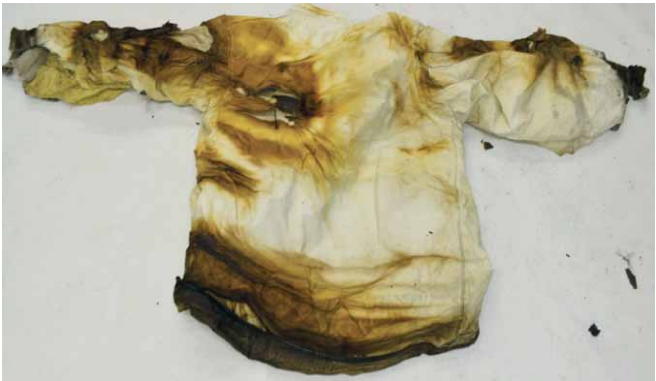
Figure 22: Substantial thermal damage visible on back of coat liner
