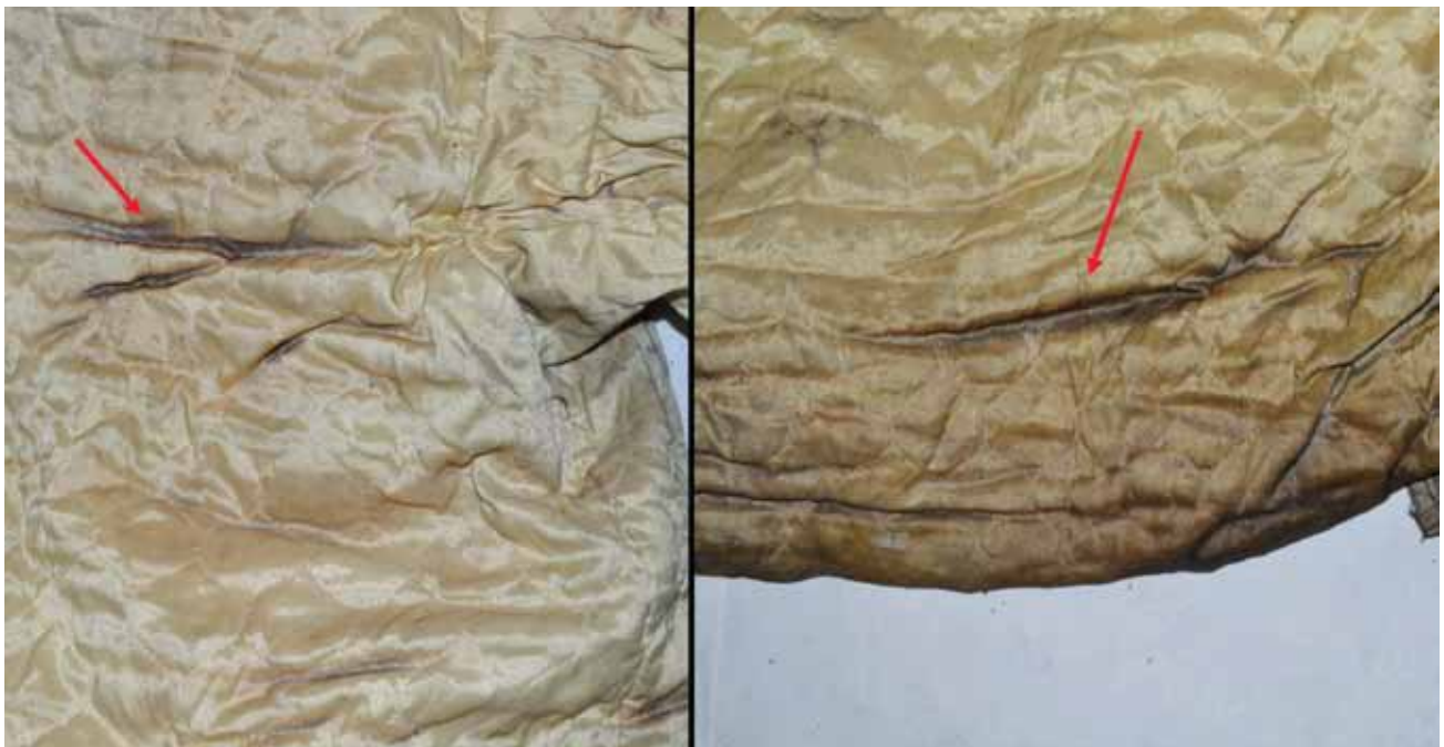
Figure 24: Close up of thermal damage to face cloth liner
