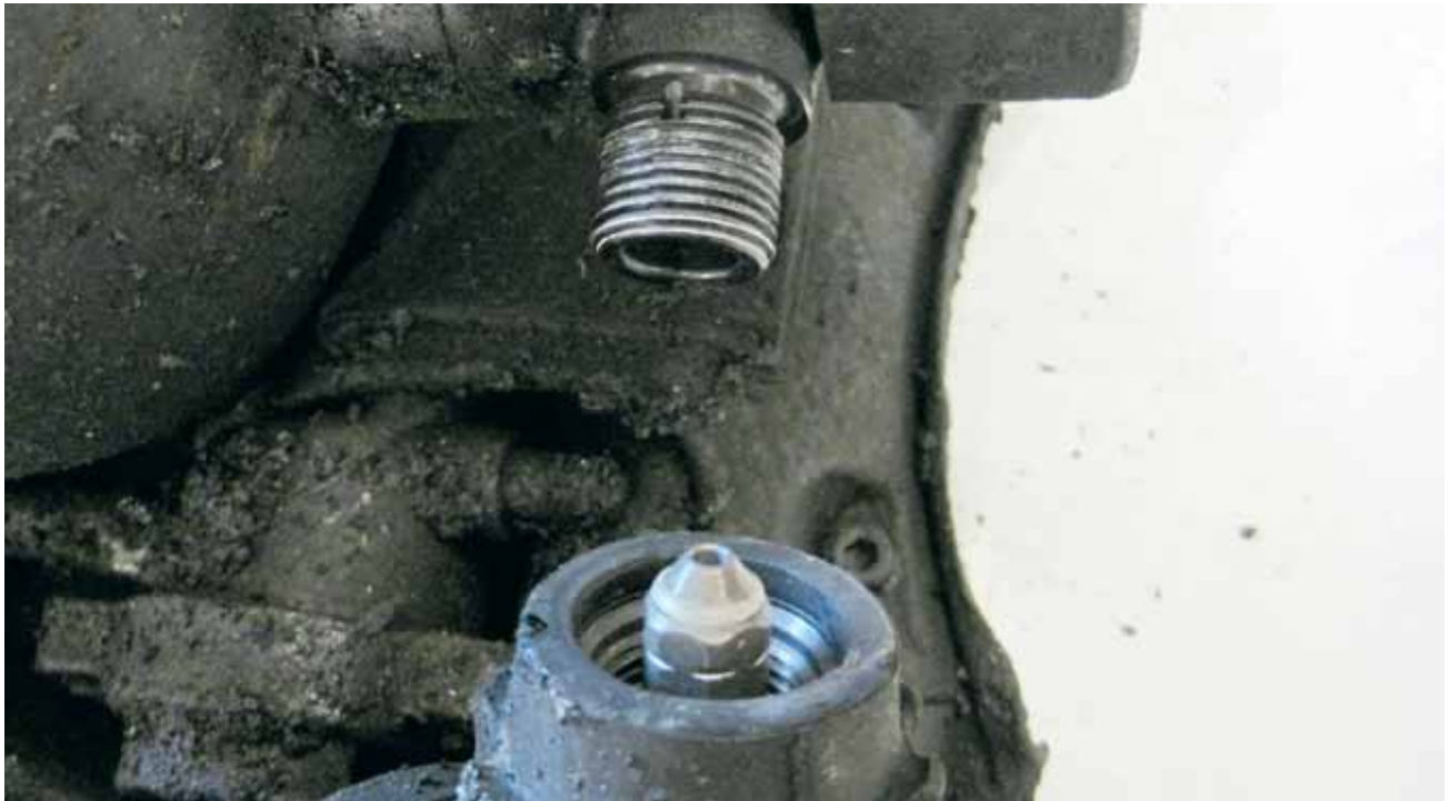
Figure 15: Cylinder attachment, o-ring and threads.
