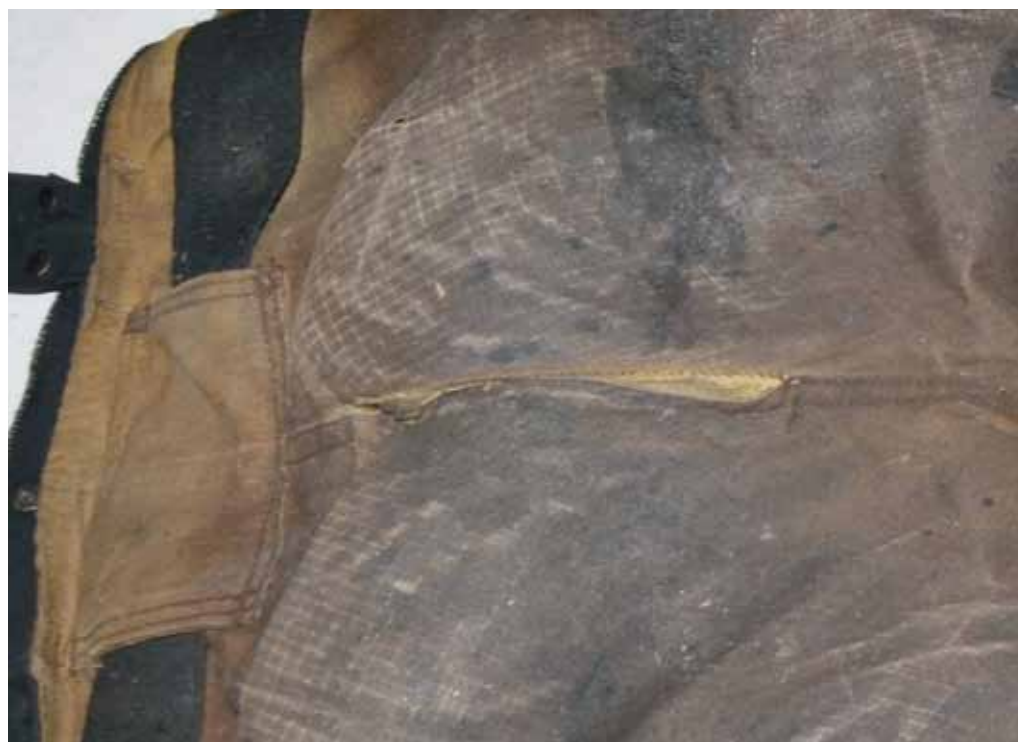
Figure 28: Seam failure in seat of pants
