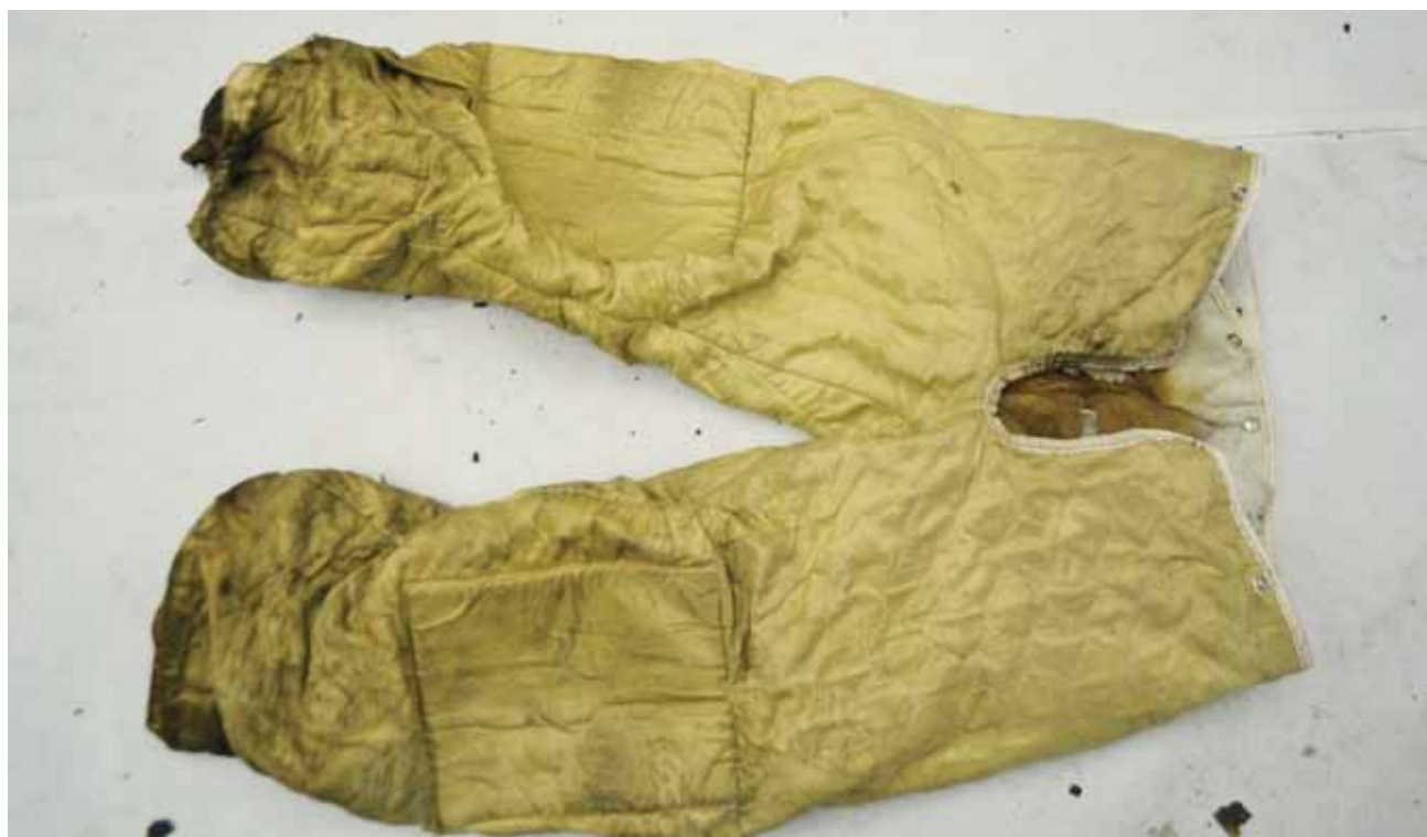
Figure 36: Liner turned inside-out showing kneepads and moderate thermal damage to cuffs
