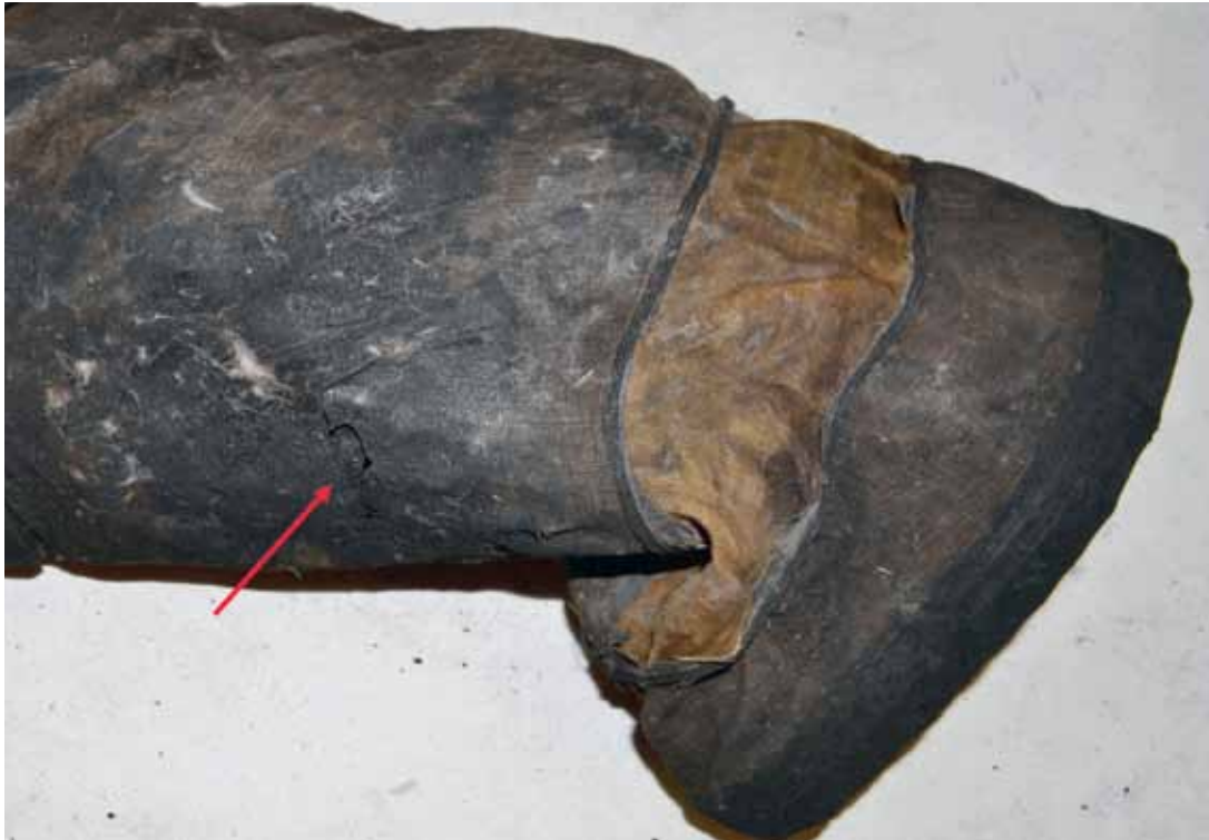
Figure 29: Thermal break open on inside of left leg and thermal damage to reflective trim on cuff
