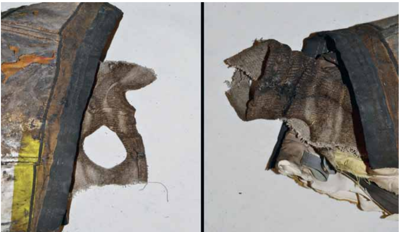
Figure 14: Substantial thermal damage on right and left cuffs and wristlets of coat
