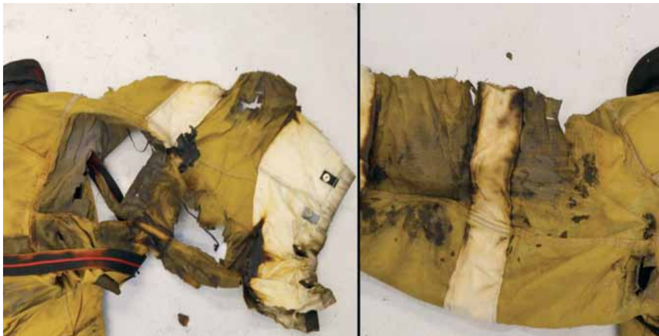
Figure 19: Close up of thermal break open on both sleeves of coat outershell
