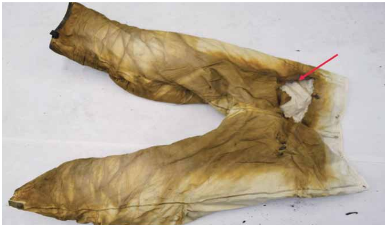
Figure 35: Thermal damage and break open in the seat of moisture barrier side of pants liner
