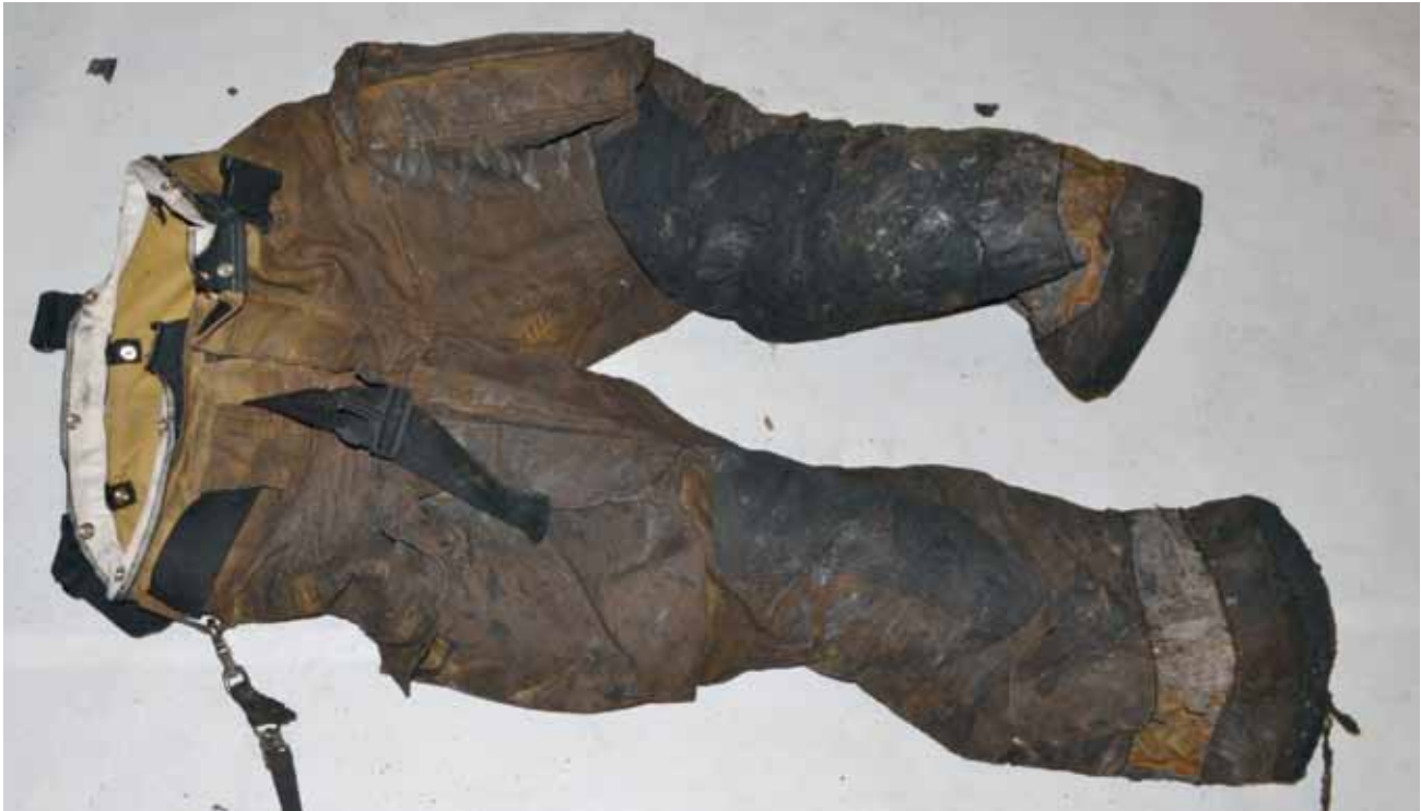
Figure 25: Substantial thermal damage to front of pants including reflective trim
