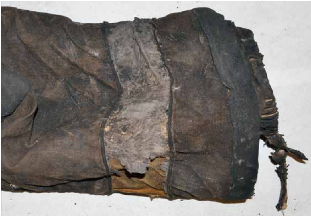
Figure 30: Substantial thermal damage visible at cuff of right leg and damage to reflective trim
