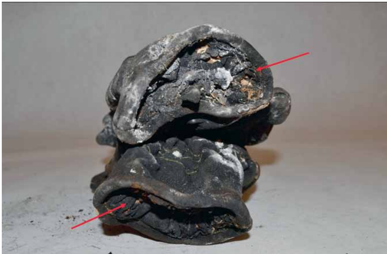
Figure 7: Substantial thermal damage extending to inside wristlet area of gloves
