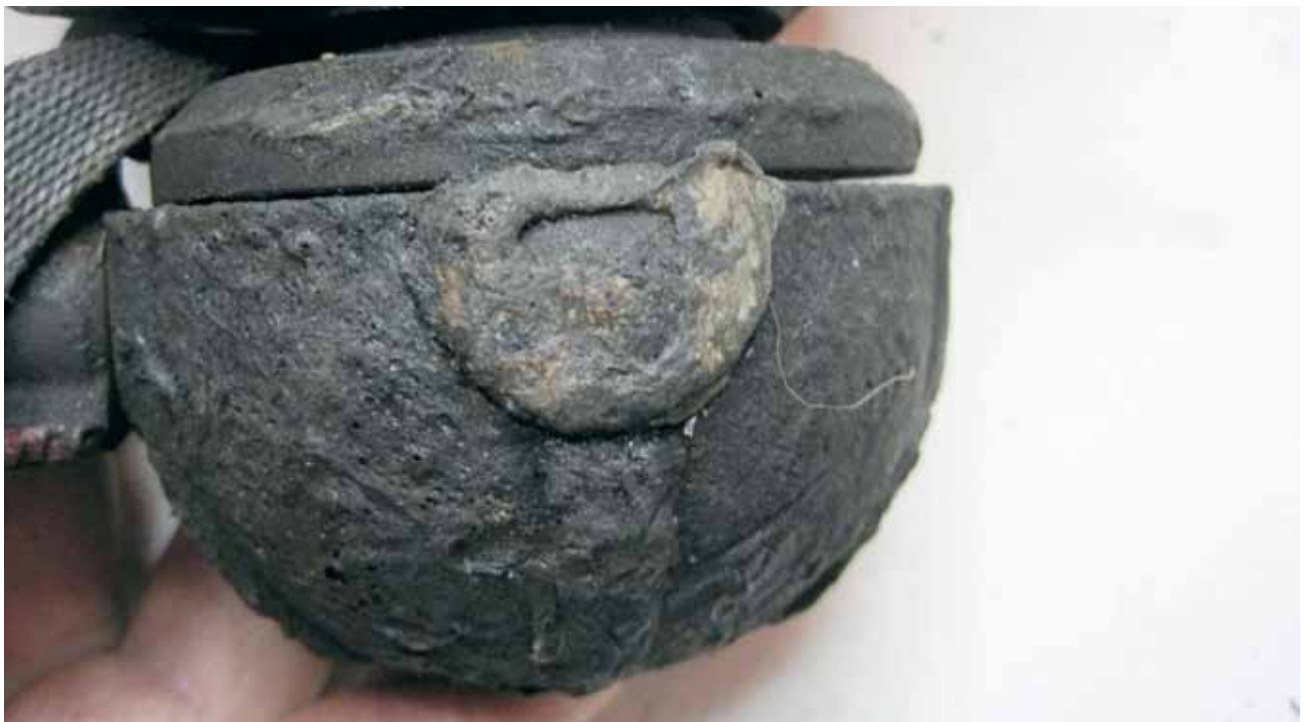
Figure 8: Melted top locking point.
