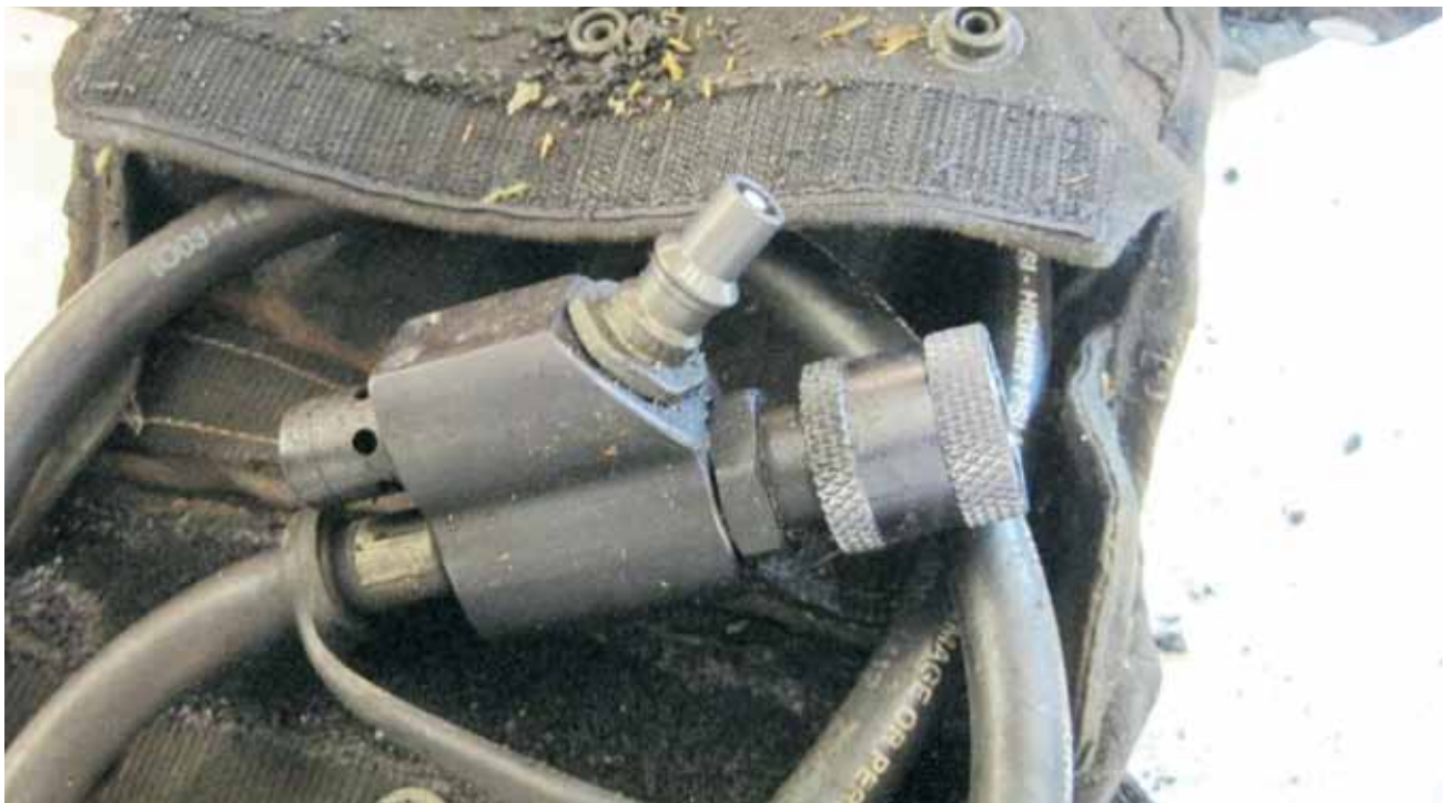
Figure 28: Both auxiliary hose fitting uncapped and clean.
