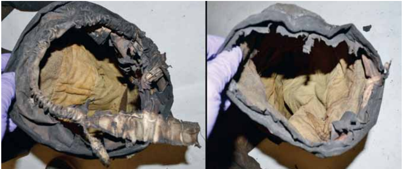
Figure 31: Substantial thermal damage to both pant cuffs and interface on left leg is missing
