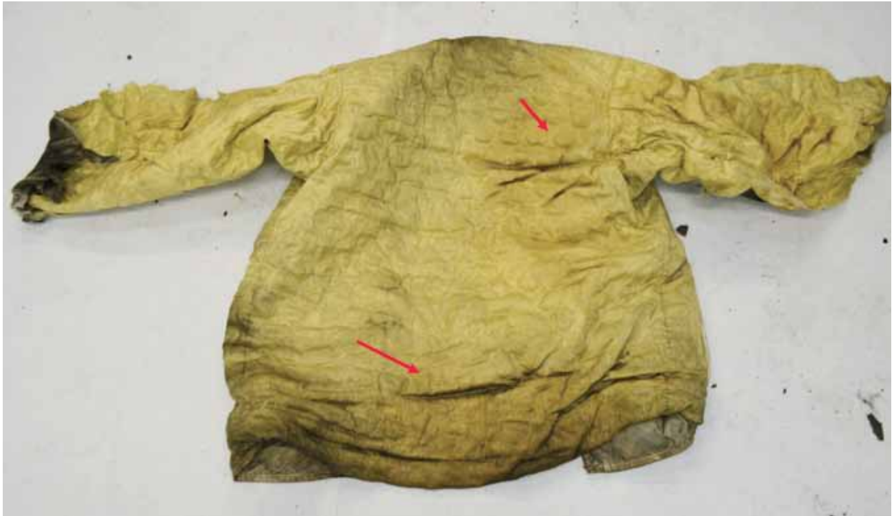
Figure 23: Liner turned inside out showing minor to moderate thermal damage to face cloth of liner
