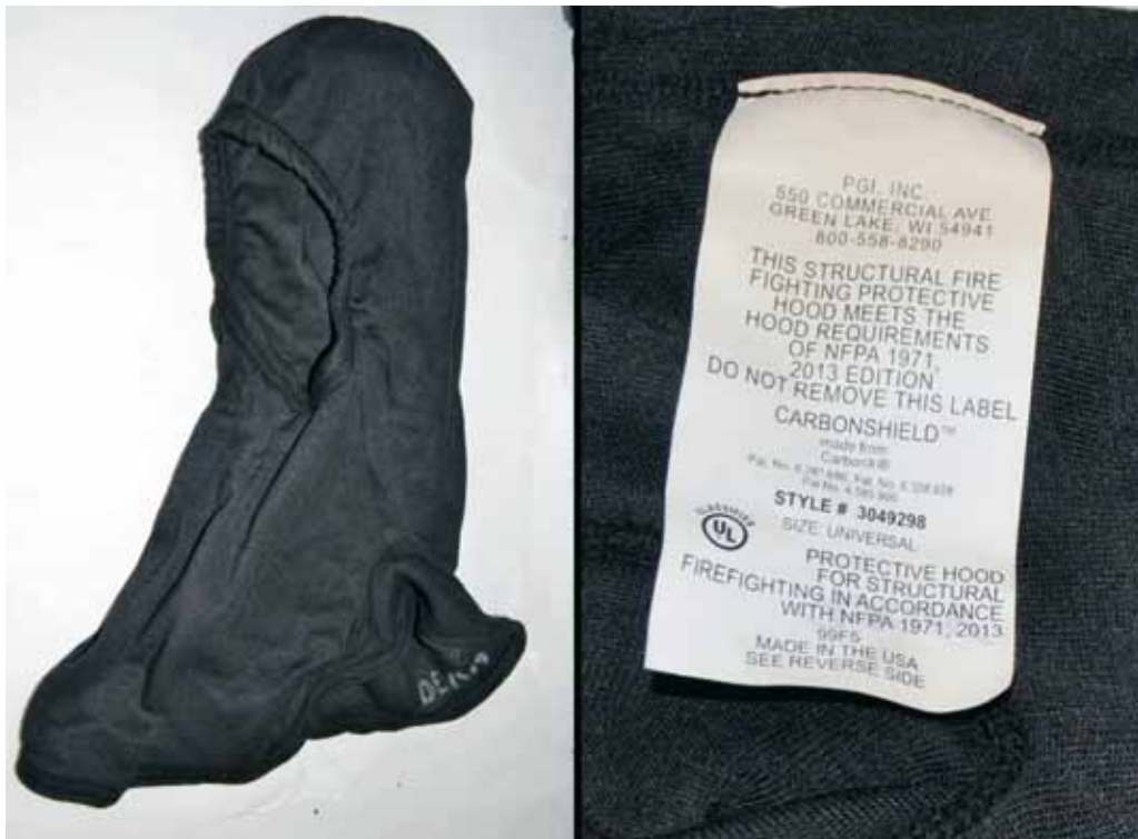
Figure 10: Hood was in good condition and certified to NFPA 1971
