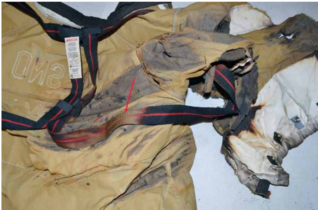
Figure 20: Dye sublimation visible on the strap of the DRD
