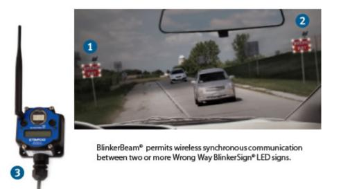
Wrong Way BlinkerSign<sup>®</sup> Warning Systems typically consist of two Wrong Way signs (1 & 2) one on each side of the roadway. When activated, the signs communicate wirelessly with each other through the BlinkerBeam<sup>®</sup> transmitter 3. Instantly both signs are flashing in unison.
