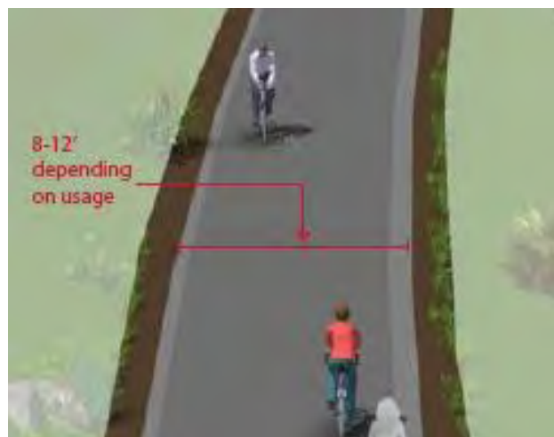
Figure 123: Surrounding land uses, environmental conditions and other factors can influence trail width.
