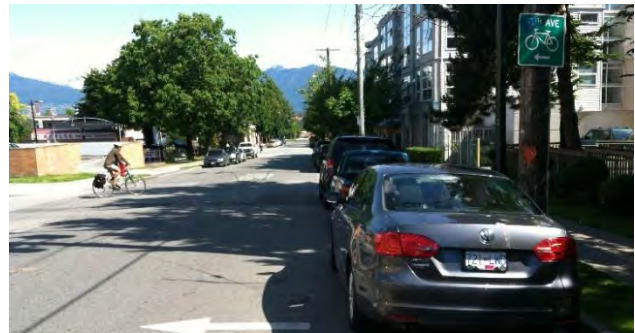
Figure 120: Turn signs are placed in advance of a turn in the bike route network.
