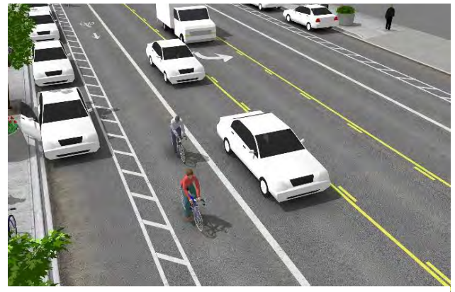
Figure 86: Buffered bicycle lanes are becoming more common throughout the United States.
