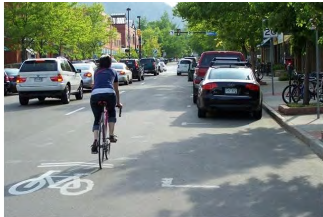
Figure 42: Shared lane markings on a two-lane, one-way street.
