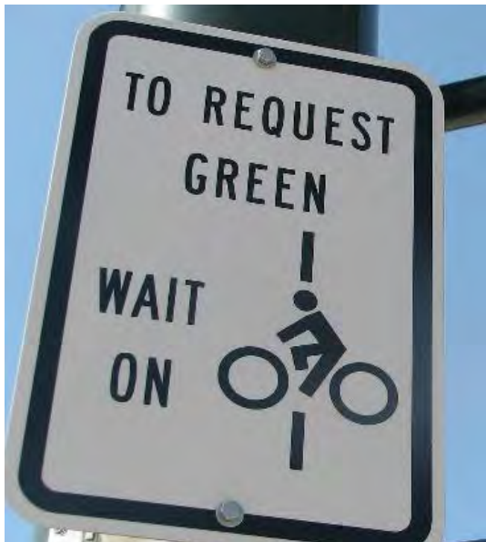
Figures 115 and 116: Signage and pavement markings direct bicyclists to use the pavement detection loop to activate a traffic signal.
