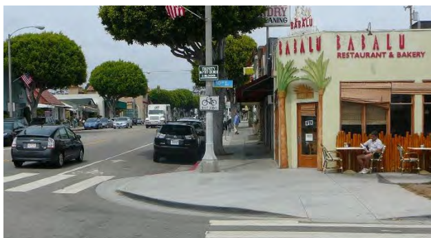
Figures 106 and 107: These curb extensions pictured above support pedestrian mobility in busy commercial districts. .
