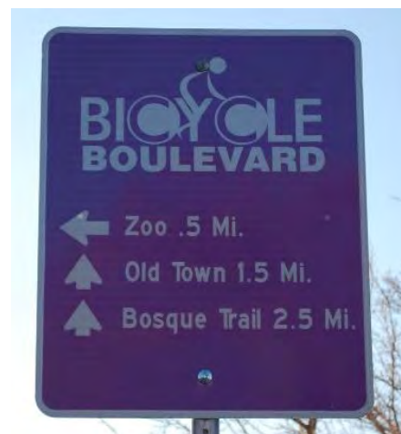
Figures 75 and 76: A combination of pavement markings and distinct signs distinguish bicycle boulevards from other shared travel lanes.
