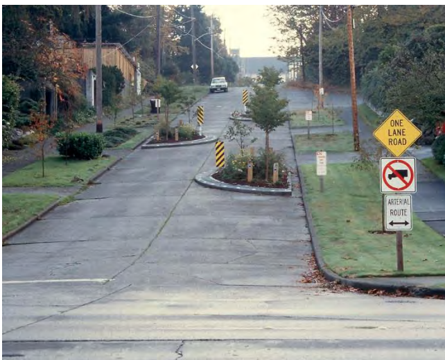
Figures 99 and 100: Chicanes slow motor vehicle traffic, creating a more calm and welcoming environment for both bicyclists and pedestrians.
