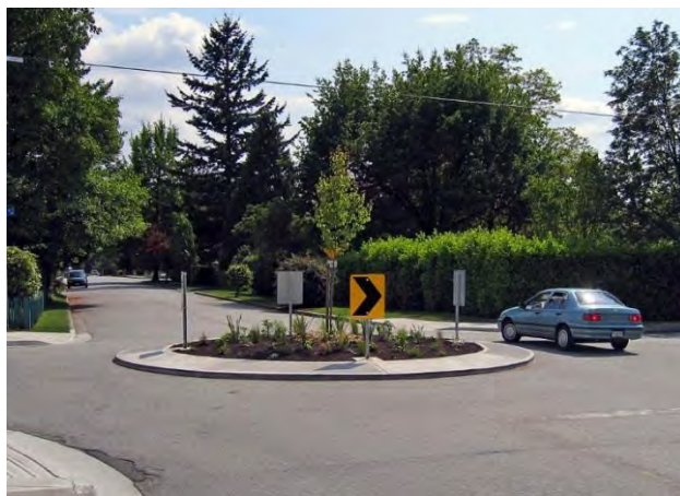
Figure 78: Traffic circles have proven to be effective intersection treatments for bicycle boulevards.
