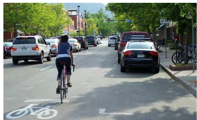
Figure 73: Shared lane markings help cyclists position themselves within the travel lane.
