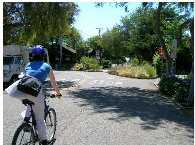
Figures 96 and 97: Traffic diverters allow through bicycle traffic while dispersing motor vehicle traffic onto adjacent roadways.
