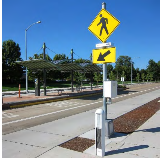
Figure 132: Rectangular rapid flashing beacons help to identify important pedestrian crossings.
