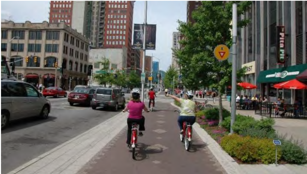
Figure 62: Complete streets take many different forms. In Indianapolis, Indiana, the Indianapolis Cultural Trail provides a cycle track to separate bicyclists from both pedestrians and motor vehicles.
