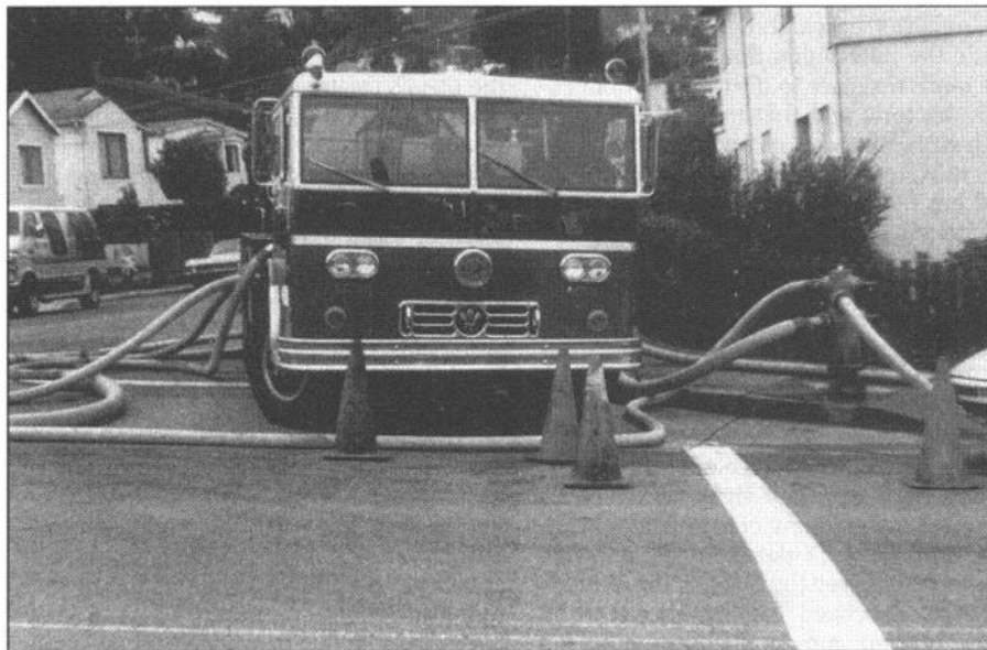
San Francisco Fire Department pumper trucks acted as makeshift booster pumps to get water to those supply areas in which numerous main breaks occurred after the earthquake Oct. 17, 1990.
