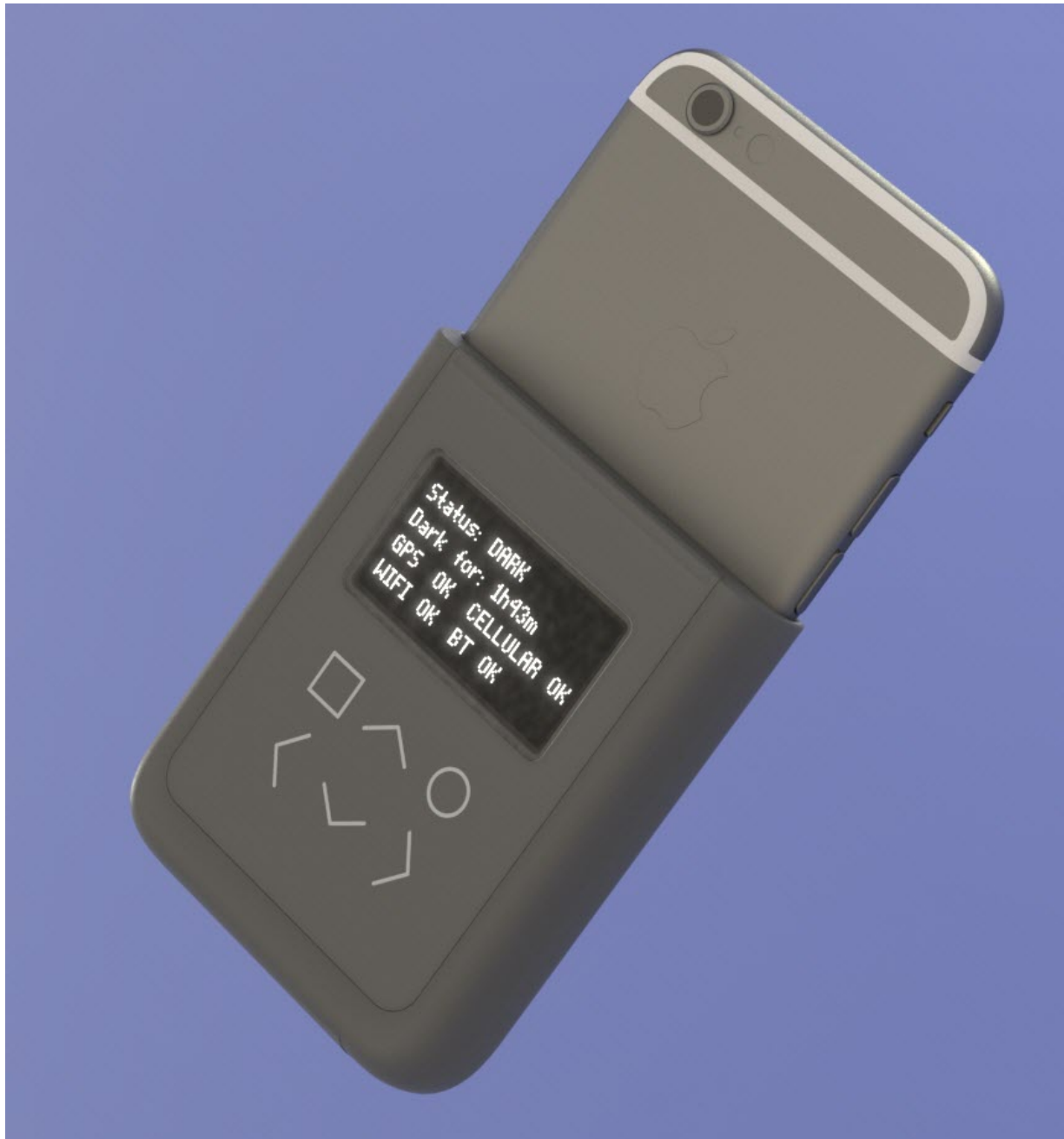
Above: Conceptual rendering of a “battery case” style introspection engine, piggybacked on an iPhone6.
