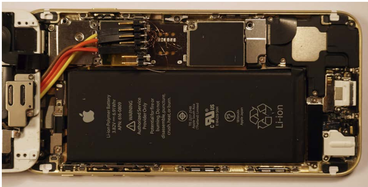
Above: image of the UART and GPS sync probing experiment. The majority of the test points are located underneath the SIM card connector, which was removed for this experiment.
