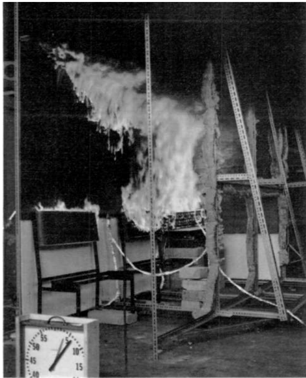
28 Involvement of second seating unit (Note flaming runnels on wall tiles)
