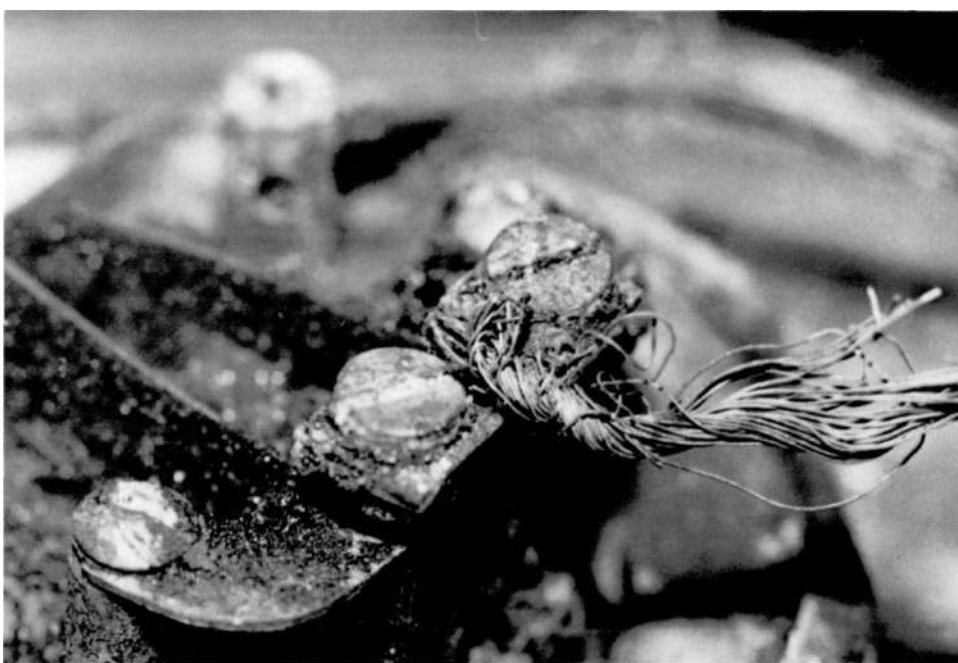
Plate 51 — Close-up photograph of same, showing poor electrical connection at the live terminal.
