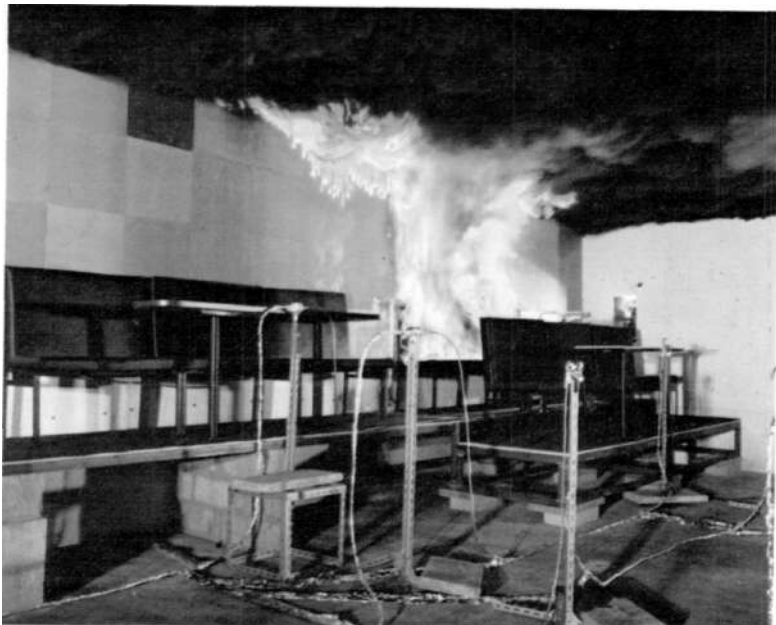
39 Lateral spread over wall tiles showing flaming runnels
