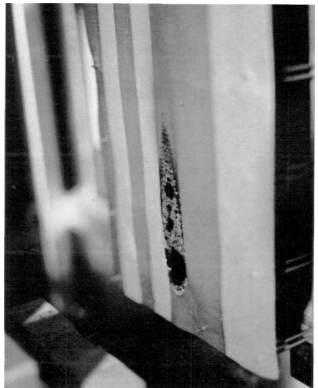
10 Limit of damage to roller blind material
