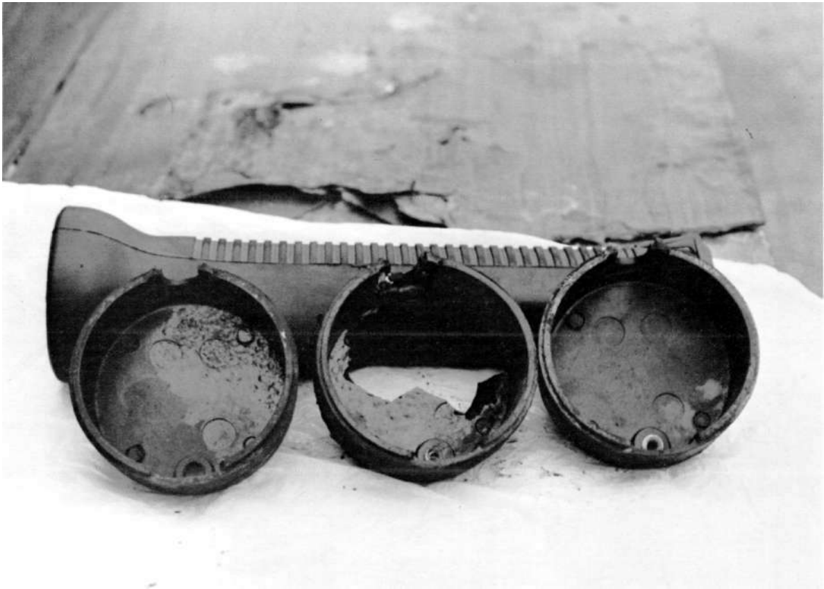
Plate 48 — Photograph of immersion heater terminal covers—interior.
