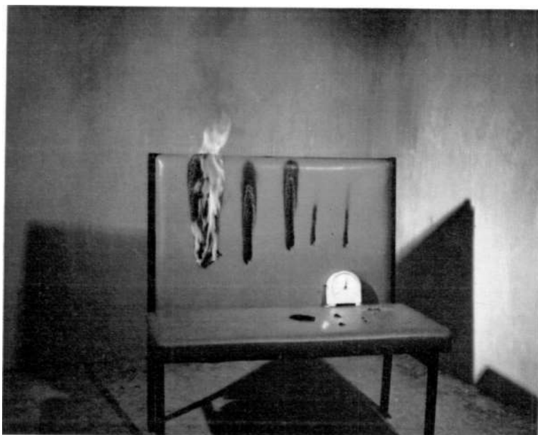
14 Larger source resulting in ignition
