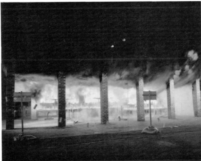
41 Fully developed fire
