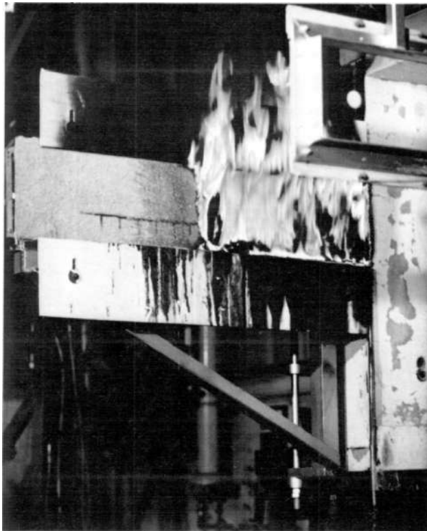
3 BS 476 Part 7 test on simulated Stateroom carpet tiles
