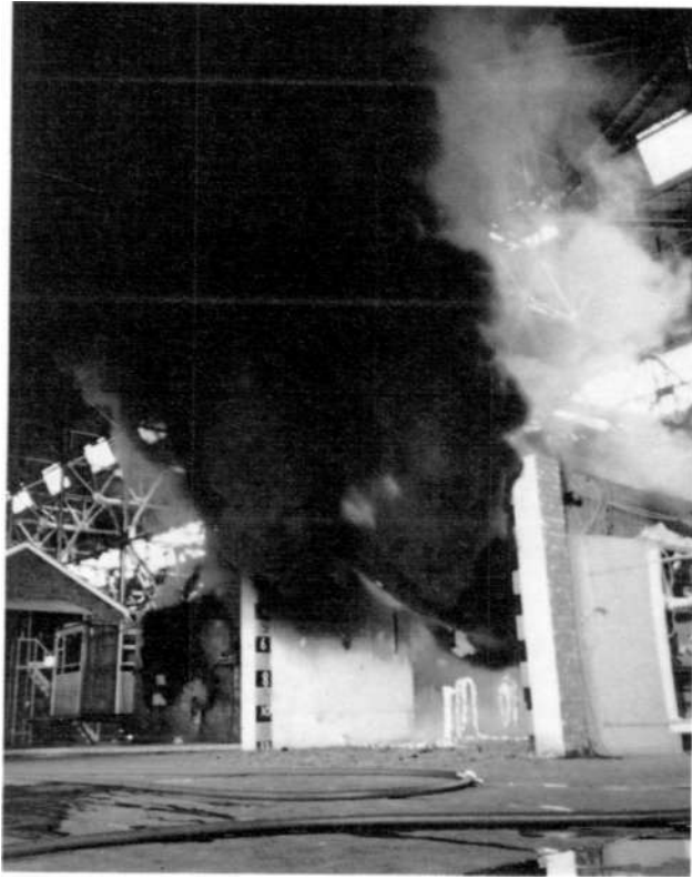
47 Smoke and flames out of exit at full fire development
