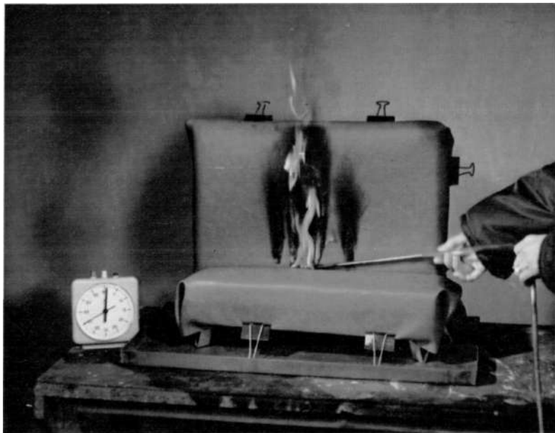
7 Ignition of test rig using source 2 of DD 58
