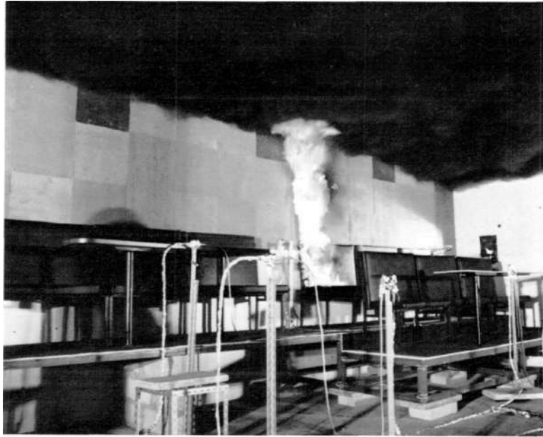
38 Fire spread up wall tiles and smoke production
