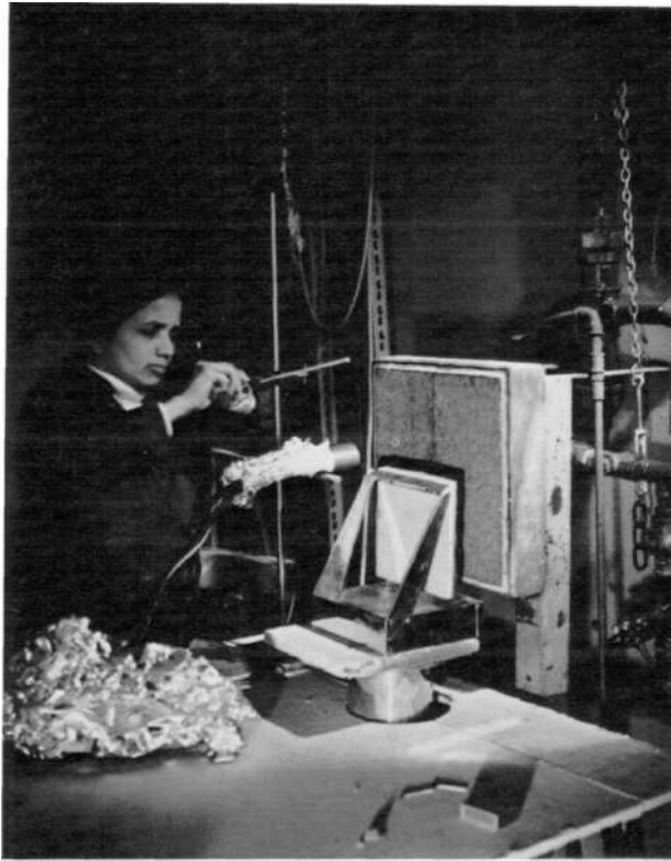
11 Radiant panel used in tests on ignition and rate of burning of carpet tiles
