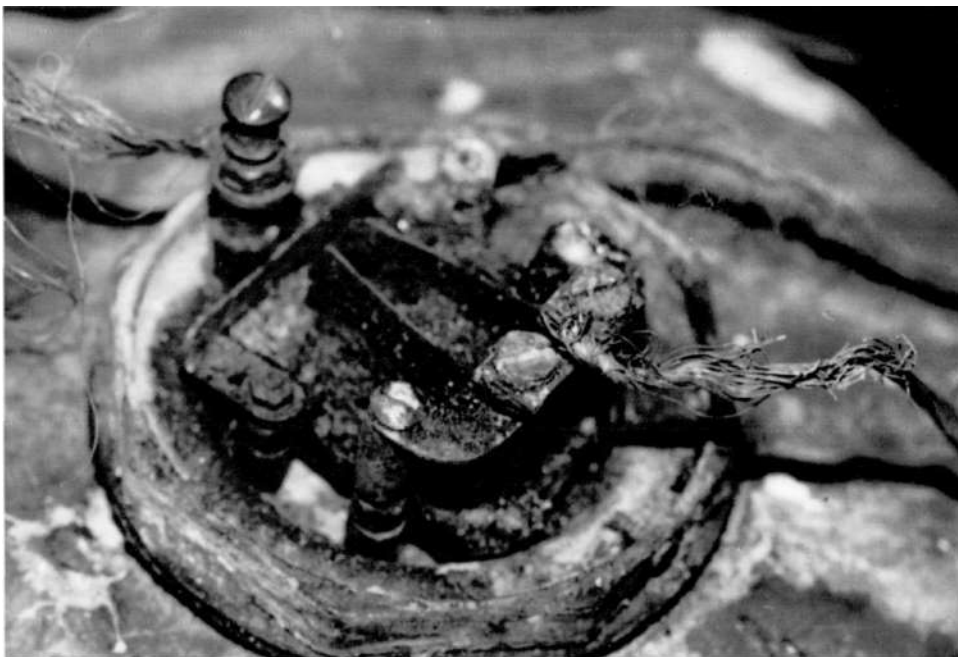
Plate 50 — Photograph showing the electrical connections at the top of the immersion heater on the cylinder in the Main Bar, taken before dismantling.
