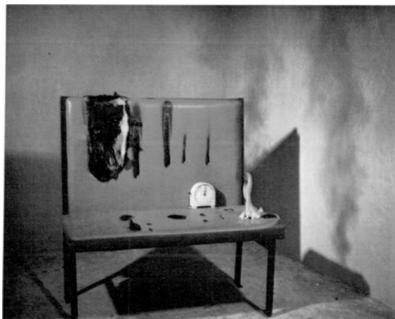
15 Ignition of seating unit by applying a match to cut surface
