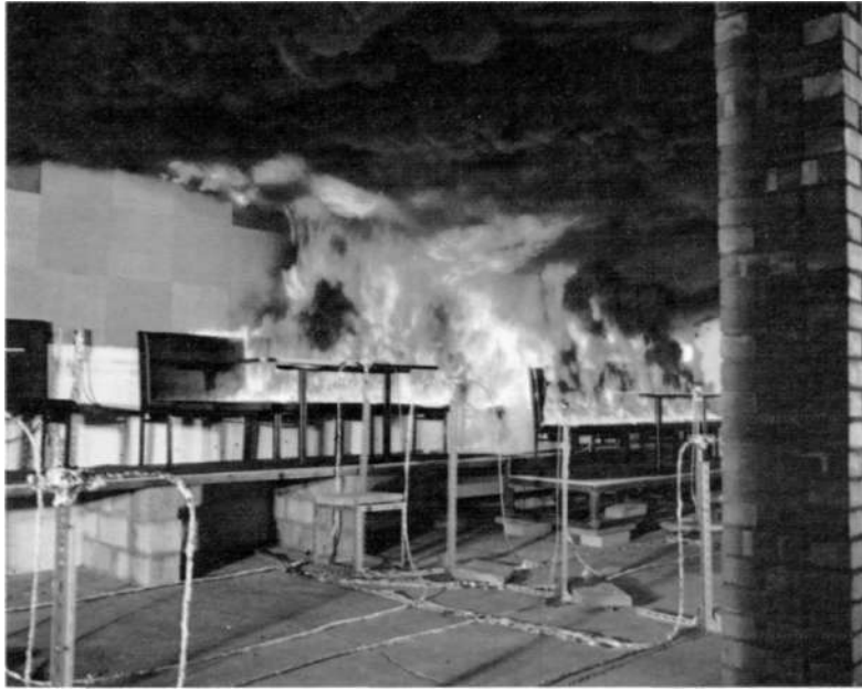
40 Lateral fire spread over second seat
