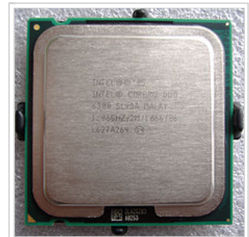
Intel Core 2 Duo – an example of an x86-compatible, 64-bit multicore processor
