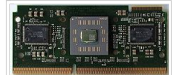
AMD Athlon (early version) – a technically different but fully compatible x86 implementation
