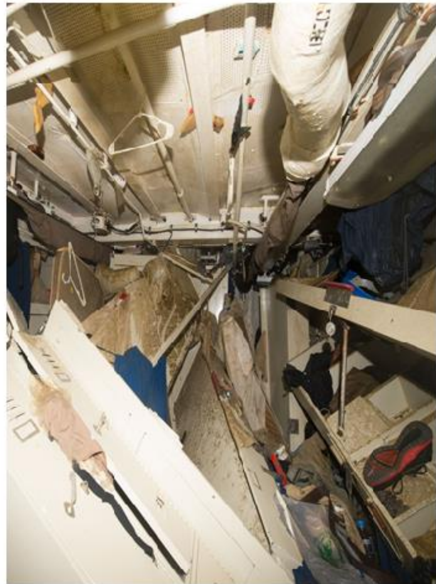
FITZGERALD Berthing 2 Racks Post-Deflooding
