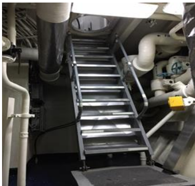
Figure 8 – Sample Berthing 2 Port Egress Ladder
