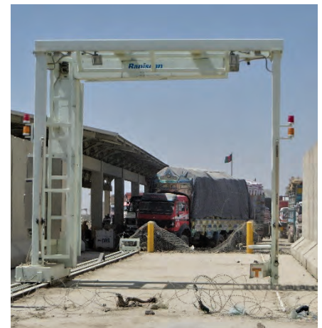
An inoperable and unused cargo scanner at the Wesh-Chaman border crossing, Kandahar Province. (SIGAR photo)
