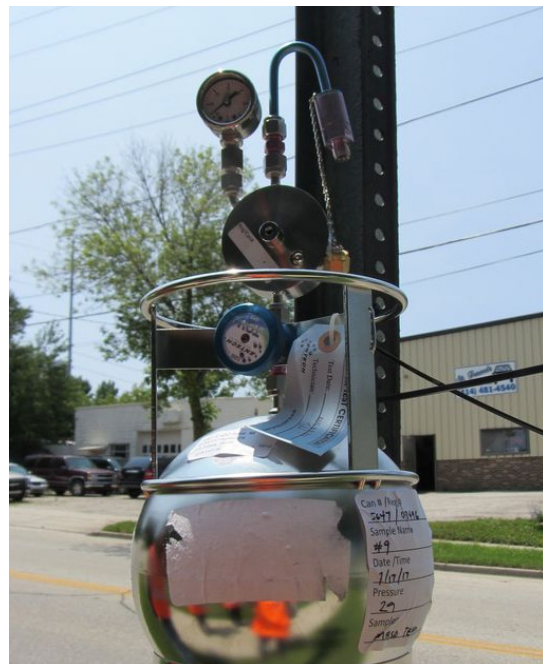
The U.S. Environmental Protection Agency tested the air outside the St. Francis facility over the summer using this canister among others.
