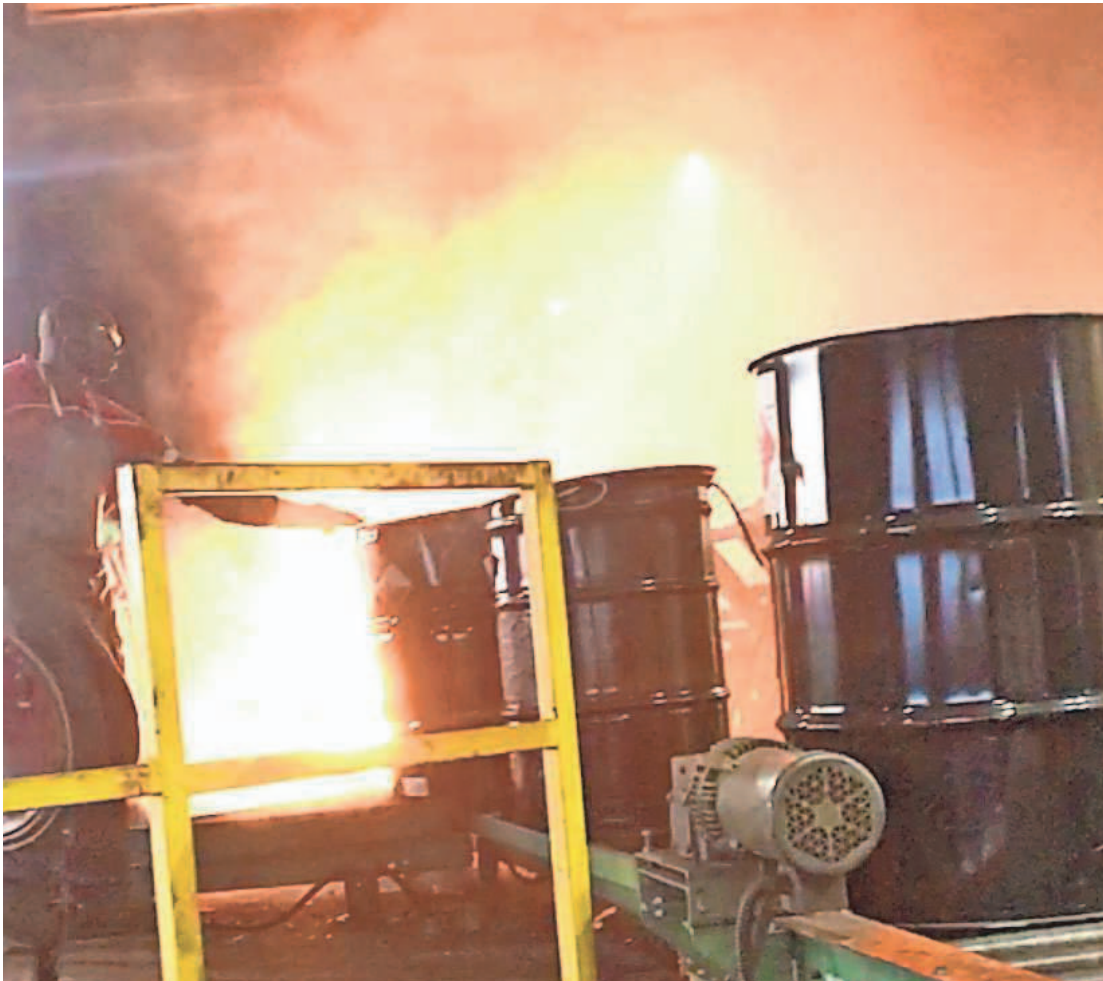
SAFETY MANAGEMENT SERVICES COMPANY AUDIT Flames burst from a burner at the Container Life Cycle Management plant in Arkansas where steel drums are refurbished. Chemicals in the bottom of the drums have caused fires that have injured workers. The photo is from a 2013 audit of the plant.
