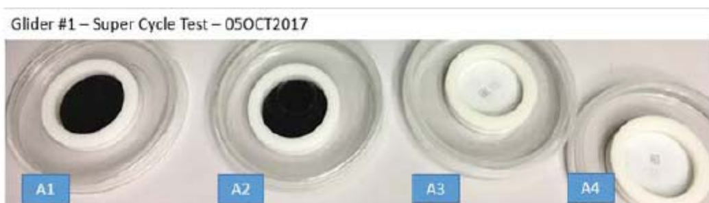
Figure 9: PM Filters from Glider #1 testing over the Super Cycle Test 2
