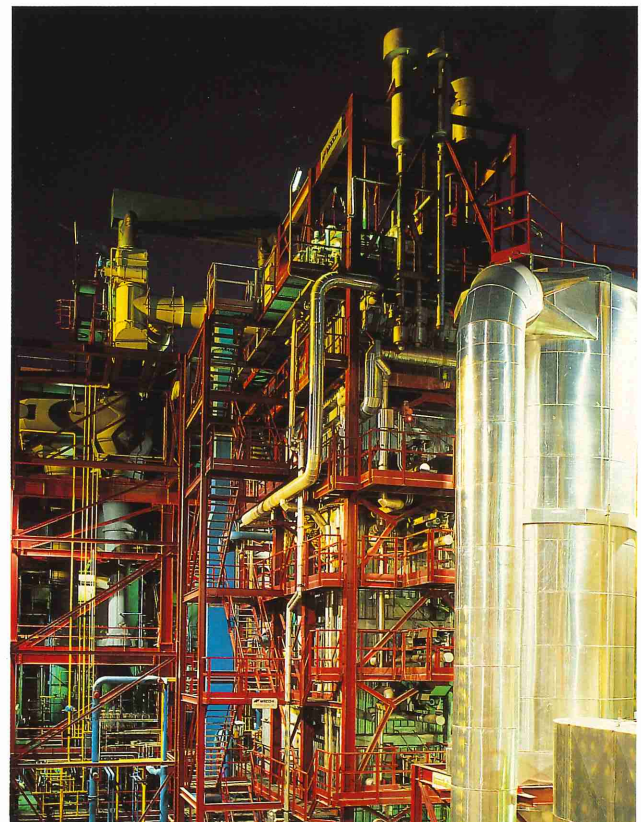
Credit: Tommaso Guicciardini/Science Photo Library TPS Termiska Processer's Commercial Gasification Plant Operating on RDF at Greve-in-Chianti, Italy
