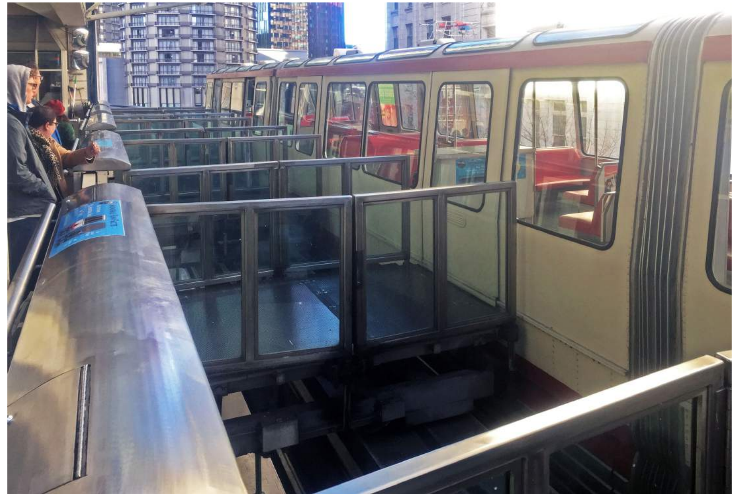
Figure 3: View of existing operable bridges to the Red Train at Westlake
