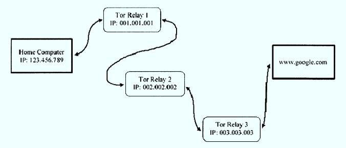
In this illustration of a Tor network connection, the website www.google.com <u>cannot</u> see the home computer IP address (123.456.789); instead it only sees the IP address of the device it is directly connected to, the third (or "exit") Tor relay, with IP address 003.003.003, which IP address cannot be traced back to the home computer user.
