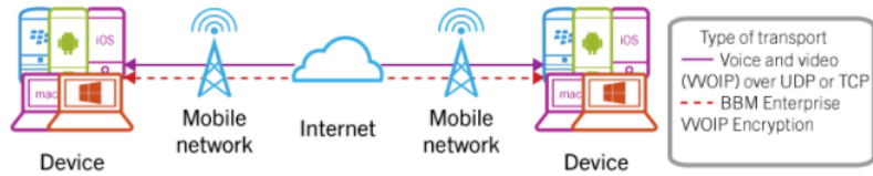
BBM Enterprise video or voice between a device on a Wi-Fi network and a device on a Wi-Fi network through the BlackBerry Infrastructure
