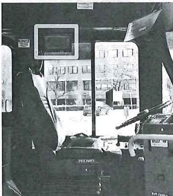
Metrobus: Transit Control Head (TCH) provides real-time schedule-adherence information, but is placed out of operator's line of sight, only allowing for use while bus is fully secured
