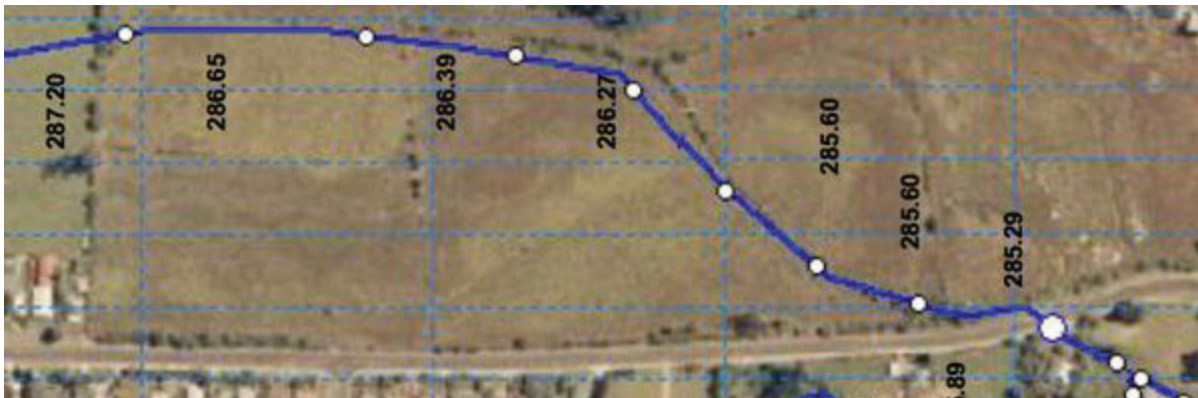
Figure 42: 100-year flood levels with PTS based on 2007 survey information (Source – BOPRC Modelling Report)
