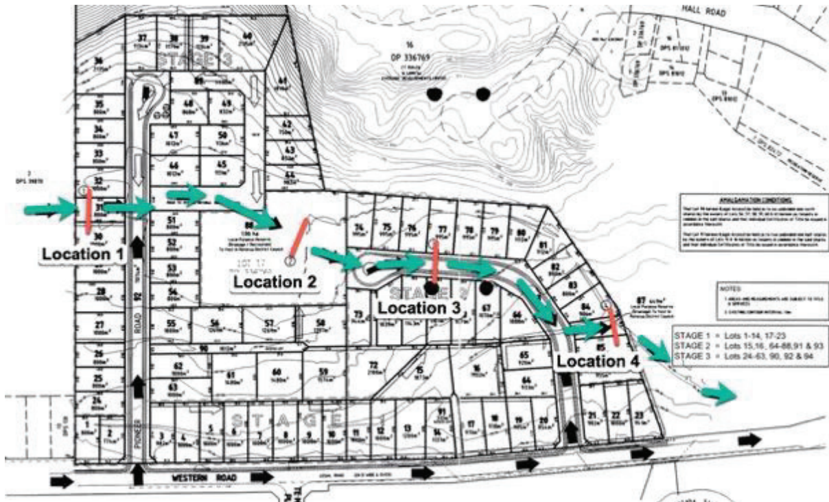
Figure 37: Outline plan of overland flow path and locations where calculations were undertaken (Source – MTEC Drawing 175781-R-P-D002 N.B. colours added by Review Panel for clarity)
