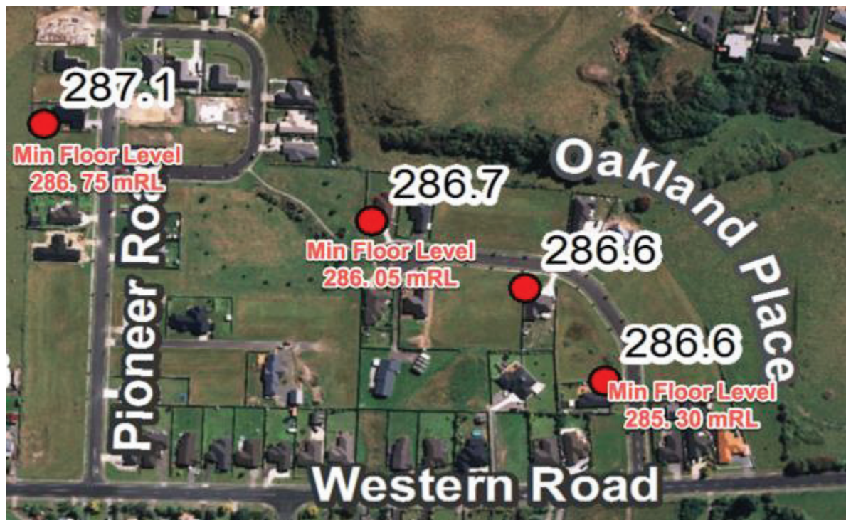
Figure 47: Figure Surveyed peak flood levels PPST April 2018 flood event (Source – BOPRC)
