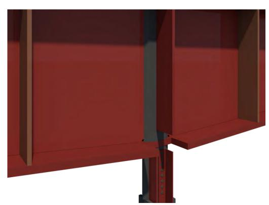
Grind the flame-cut surface of the web hangers to a smooth surface, and Magnetic Particle test.
