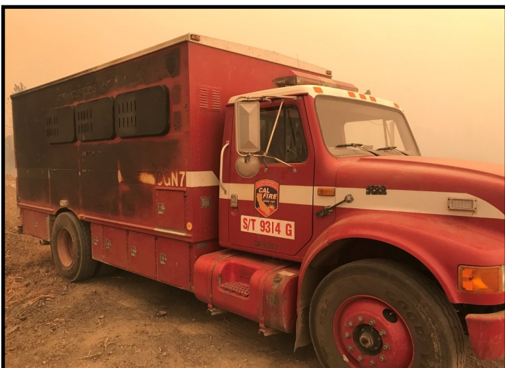
Example of damage to crew carriers in the TRA near DP-25.
