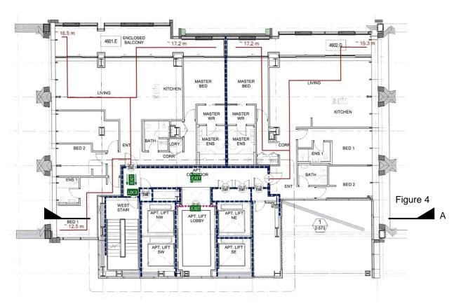
Figure 1: Plan L46 – showing 'half floor' apartments with connecting lobby between the lifts and West stair (not to scale)
