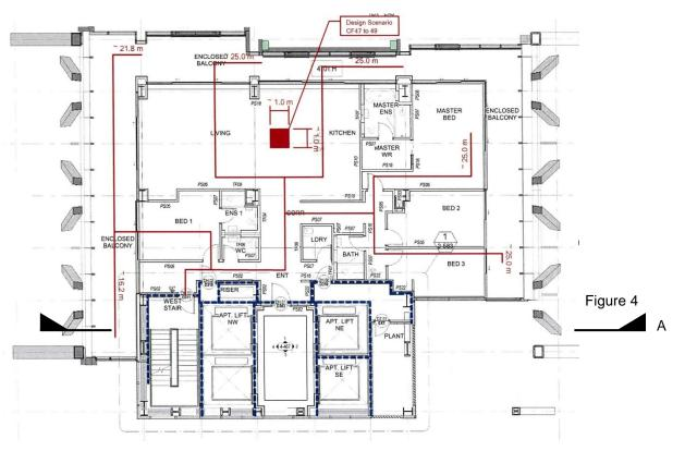
Figure 2: Plan L47 – showing 'full floor' apartment with no connecting lobby between the lifts and West stair (not to scale)
