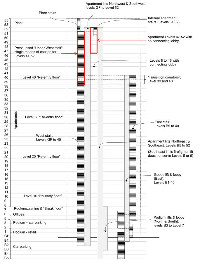
Figure 4: Schematic of lifts and stairs: Elevation A-A
