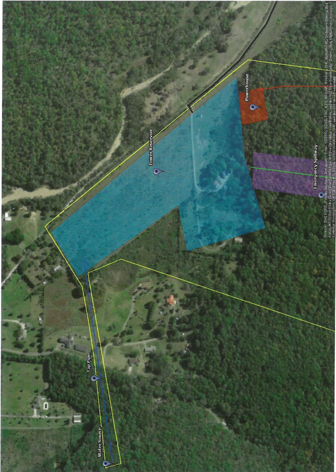
4.3.1: Freestone Project Lower Reservoir with Tap Pipe and Water Source
