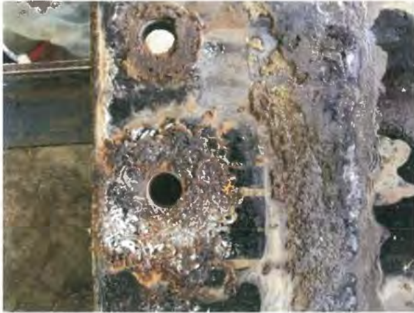
Figure 14 Swarf between drawbeam and truck side plates
