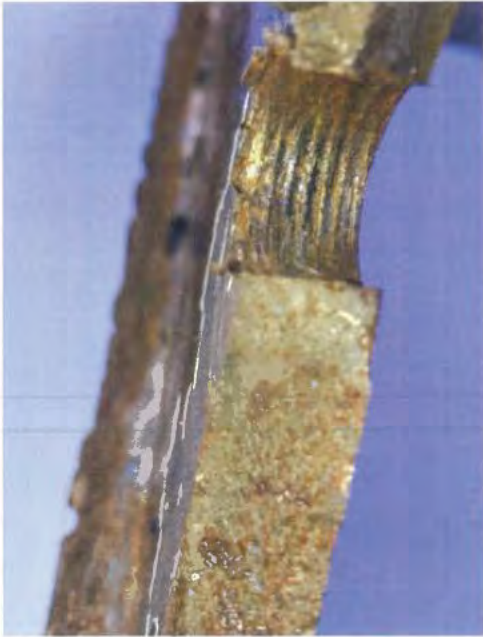
Figure 10 Thread bearing marks
