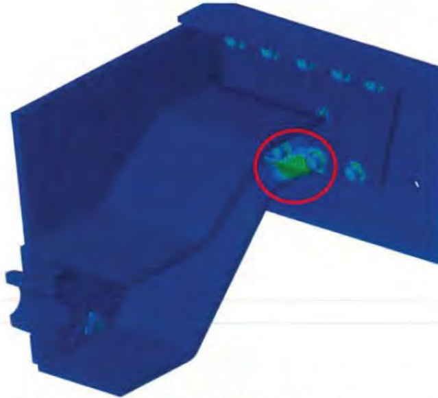
Figure 40 Residual stress from 110kN load, red circle
