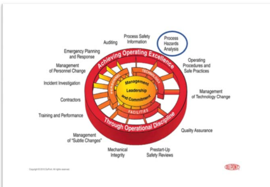
Figure 24. Where PHA is Located on DuPont’s Process Safety Management and Risk Model (PSM Wheel) [54, p. 2]. Source: DuPont, with annotations by CSB.
