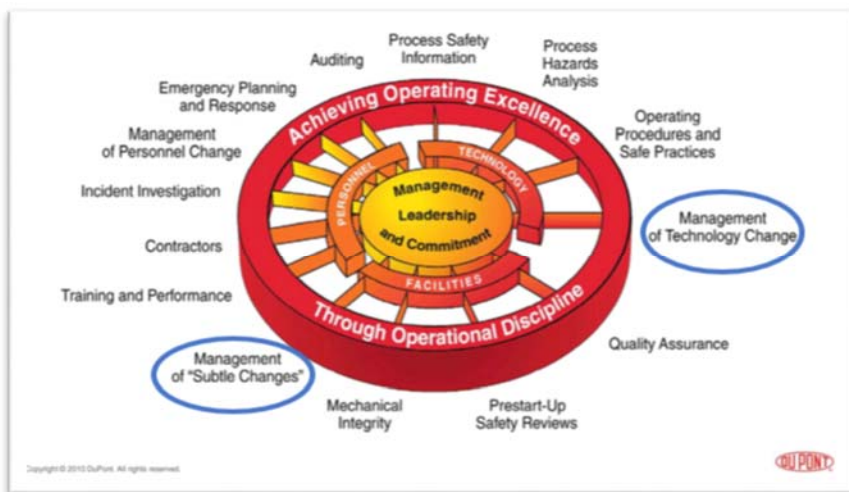
Figure 29. Where MOC is Located on DuPont’s PSM Wheel [54, p. 2]. Source: DuPont, with annotations by CSB.
