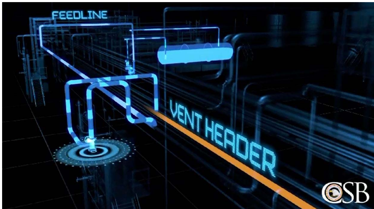
Figure 32. Excerpt from CSB Animation. It depicts the piping arrangement that allowed liquid methyl mercaptan from the feed line (blue) to flow into the waste gas vent header piping (orange). Source: CSB.
