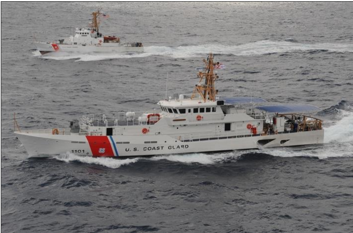
Figure 6. Fast Response Cutter With an older Island-class patrol boat behind
