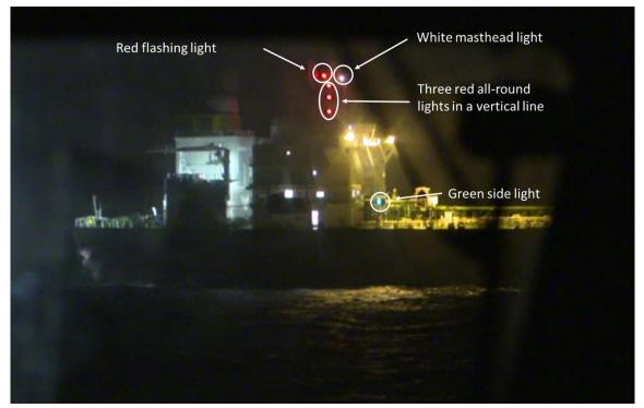
Figure 35: The lights exhibited abaft midship on Sola TS, viewed from the starboard side during the observation voyage. Photo: The police
