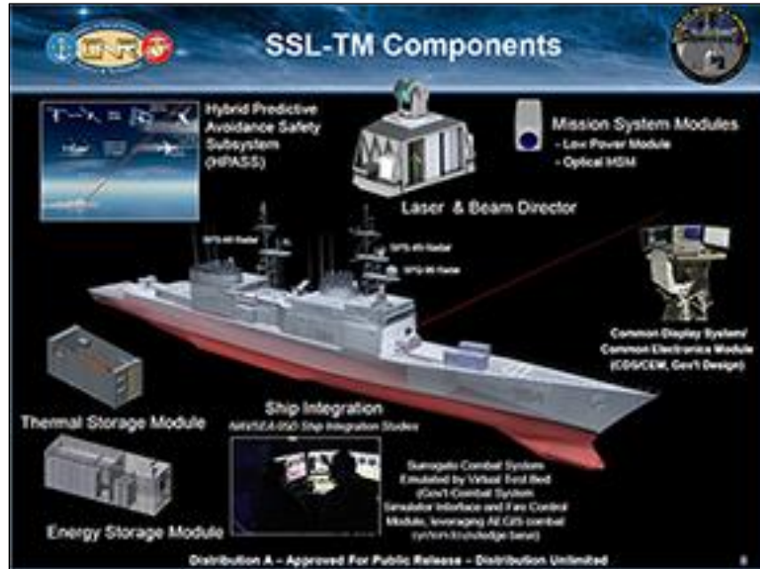
Figure 4. ONR Graphic of SSL-TM Laser System Artist's rendering of installation on Navy's Self Defense Test Ship
