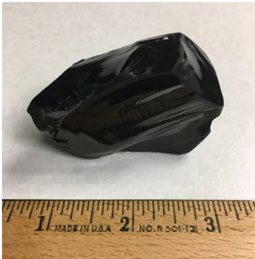
Figure ES-2. Treated simulated HLW. Sample of simulated HLW that has been mixed with a glass-forming silica mixture at high temperature and then cooled into a glass form—a process called “vitrification.” (Source: NWTRB)
