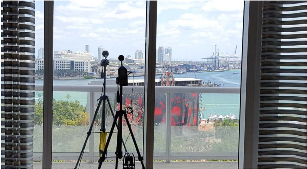
Figure 1, k. Short Term Test Position 4 - Informal party room (10th floor pool deck). Analyzer on tripod. Long term monitor visible on balcony. Ultra main stage visible.
