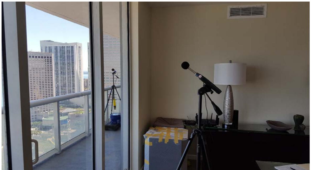
Figure 1, c. Short Term Test Position 1 - Unit 2802 dining room. Analyzer on tripod. Long term monitor visible on balcony.
