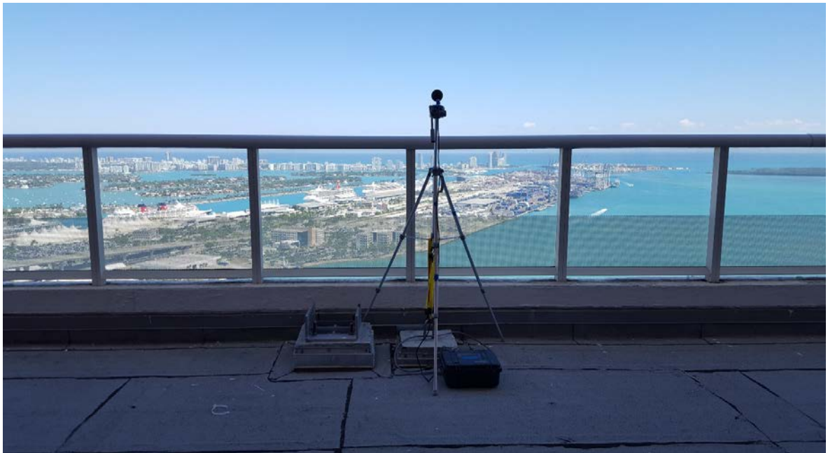
Figure 1, e. Long Term Test Position L2 - building roof (55th floor).
