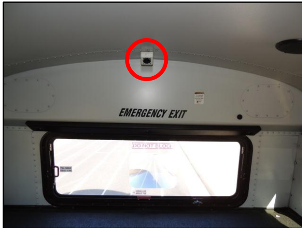
Figure 24: Surveillance camera in the back of the bus.
