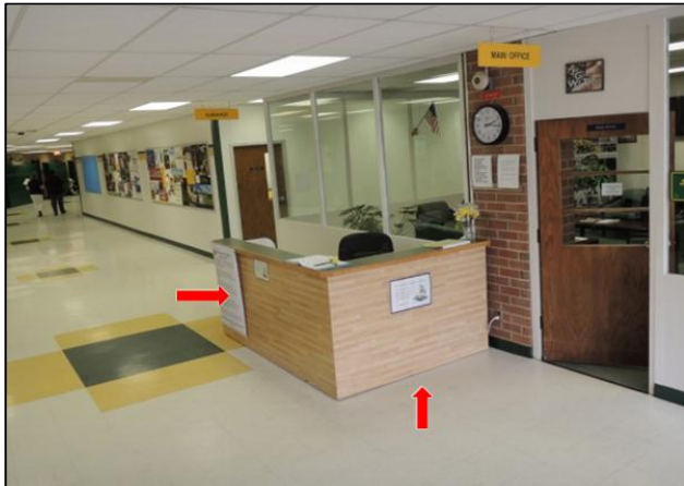
Figure 12: Red arrows indicate ballistic steel plating.
