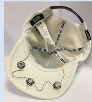
(U) Research version of hat with light emitting diodes (LEDs). 8
