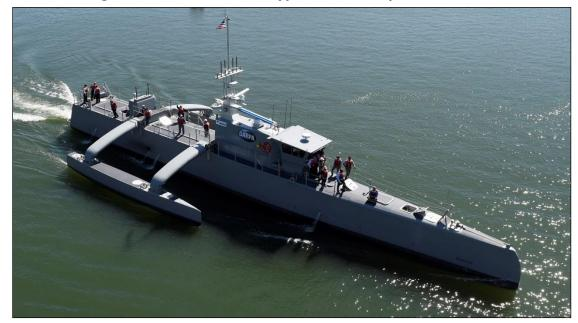
Figure 5. Sea Hunter Prototype Medium Displacement USV
