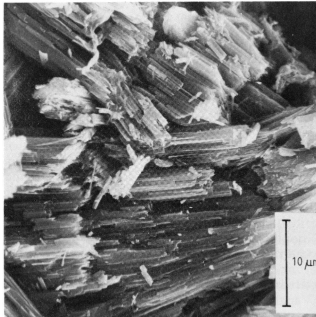
Plate 1 : Scanning Electron Microscope image of erionite crystals from the Kaipara Harbour erionite deposit. Photo from L.P. Aldridge and C.G. Pope 'Infrared and absorption studies of a New Zealand erionite.' New Zealand Journal of Science , vol 24, pp 263-271 (1981).
