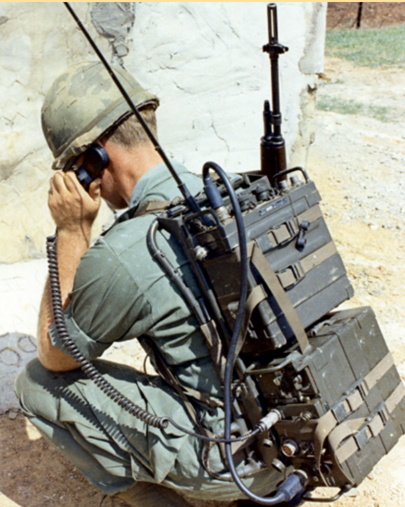
The NESTOR system was developed in answer to the military's need for lighter and more efficient communication systems. The Soldier above is using the KY-38 "manpack."
