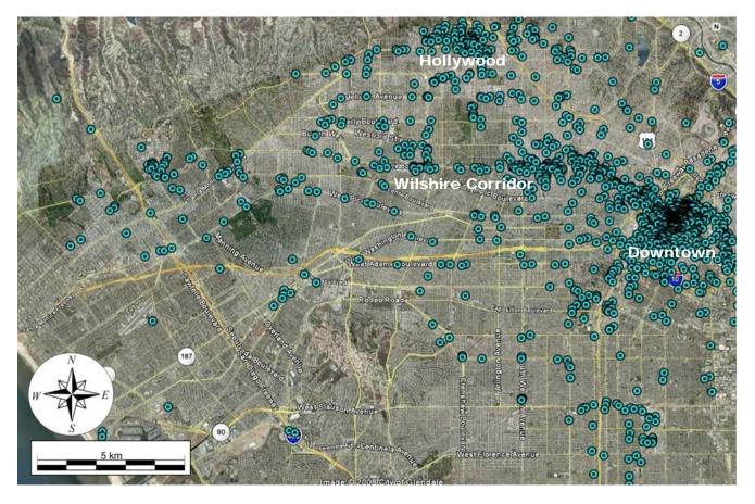
Figure 2. Subset of nonductile concrete inventory overlaid on image of Los Angeles.
