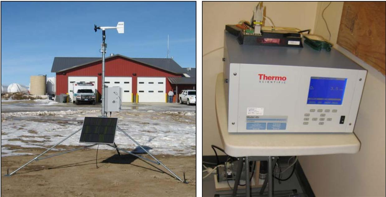
Figure 2-1. Tripod with Air Toxics Canister and Sorbent Cartridge Media and Meteorological Monitoring Equipment (left) and an Ozone Monitor at an Interior Location Nearby (right).
