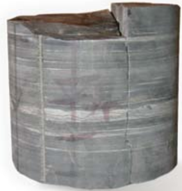
Core from organic Devonian shale formation
